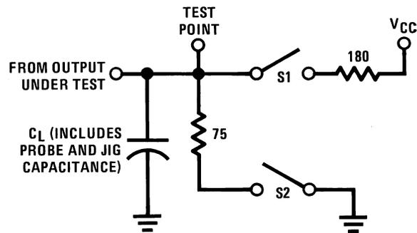
S1 and S2 of load circuit are closed except where shown.
