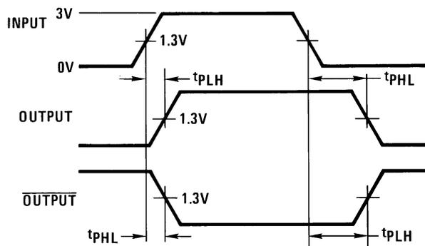
$f = 1 \text{ MHz}, t_r \leq 15 \text{ ns}, t_f \leq 6 \text{ ns}$
