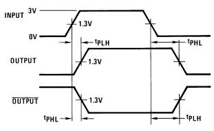
$f = 1 \text{ MHz}, t_r \leq 15 \text{ ns}, t_f \leq 6 \text{ ns}$
