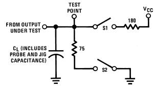
S1 and S2 of load circuit are closed except where shown.
