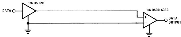
Figure 7. Single Wire with Driver Ground Reference—RS-423
