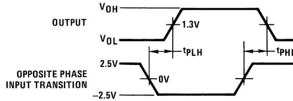
Diagram shown for  $\overline{\text{ENABLE}}$  low.
