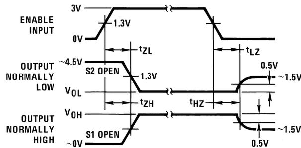
S1 and S2 of load circuit are closed except where shown.
