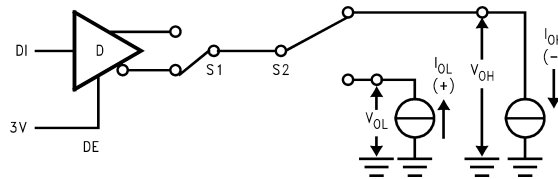
Figure 4. Driver V_{OH} and V_{OL}
