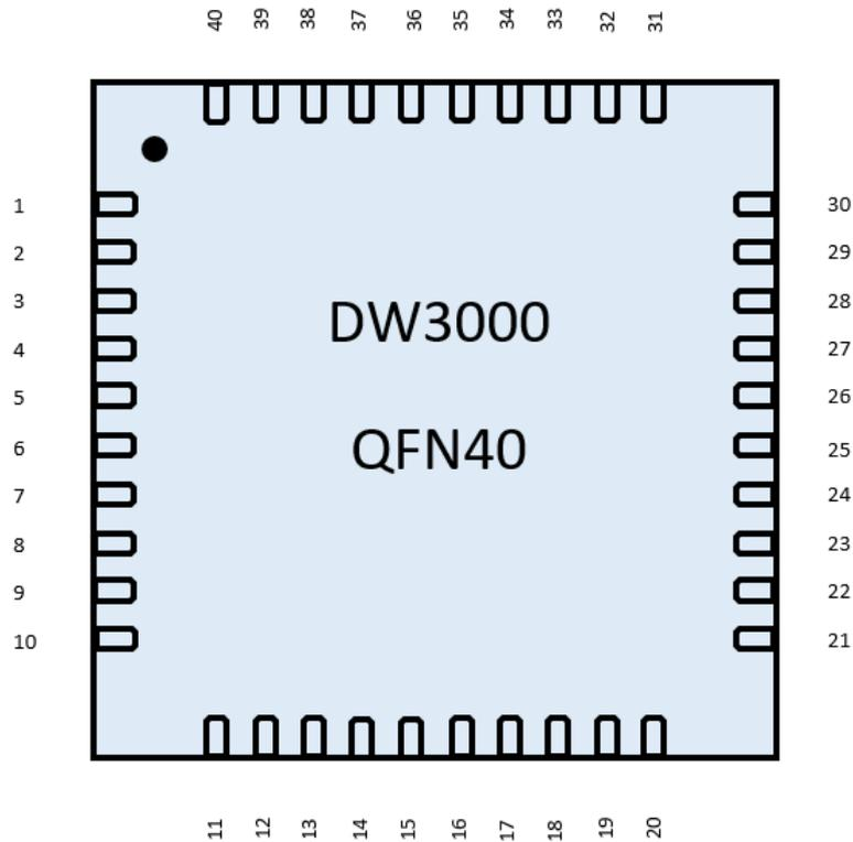
Figure 2: The QFN Top view pin assignments
