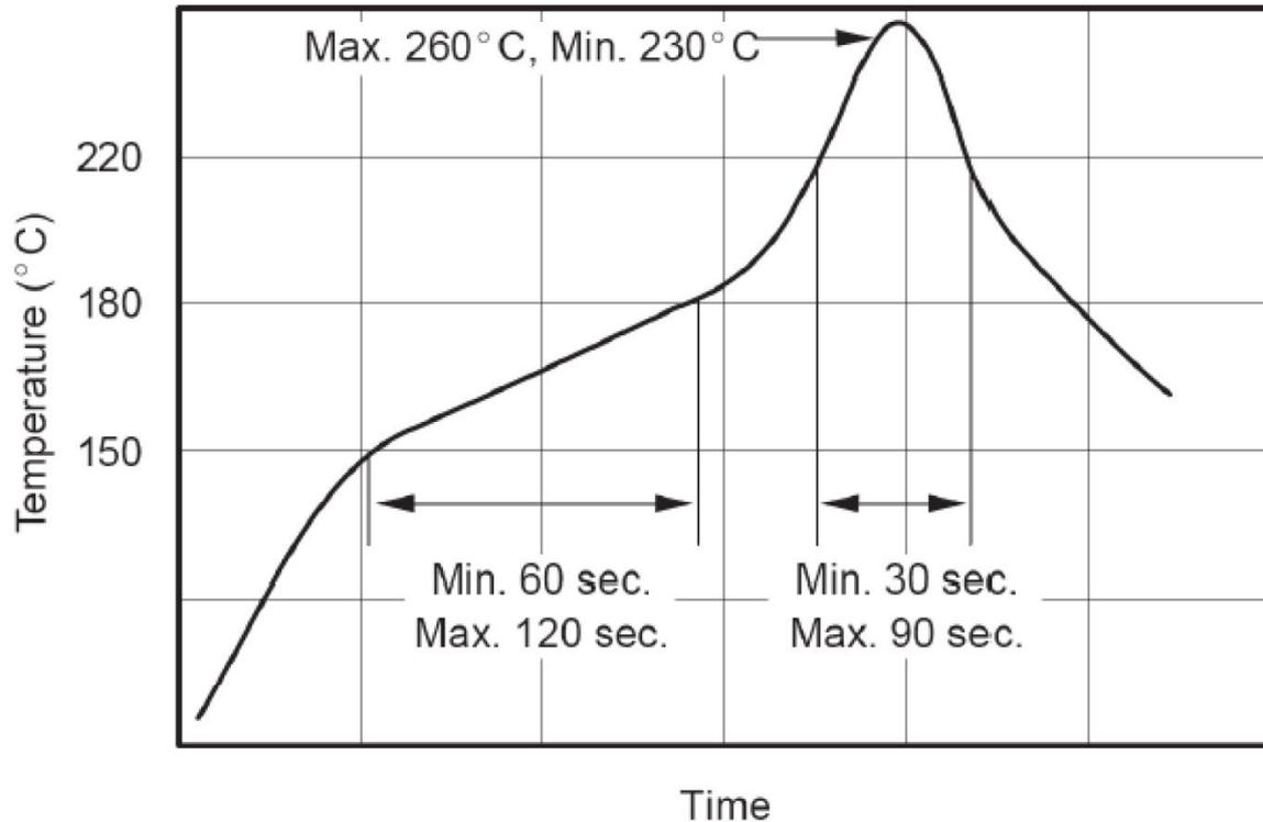
Figure 36 Reflow Profile of the WLCSP package
