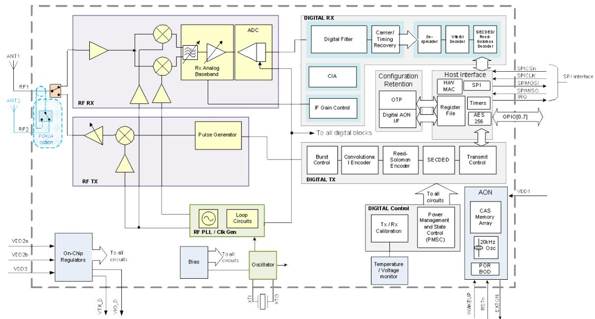
**Figure 1: IC Block Diagram**
