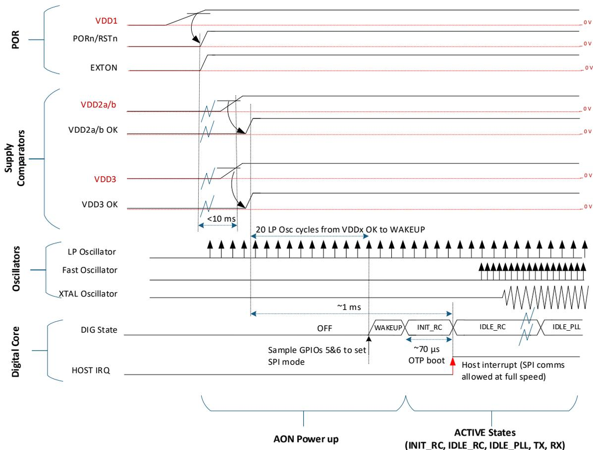
Figure 21: Timing diagram for cold start POR
