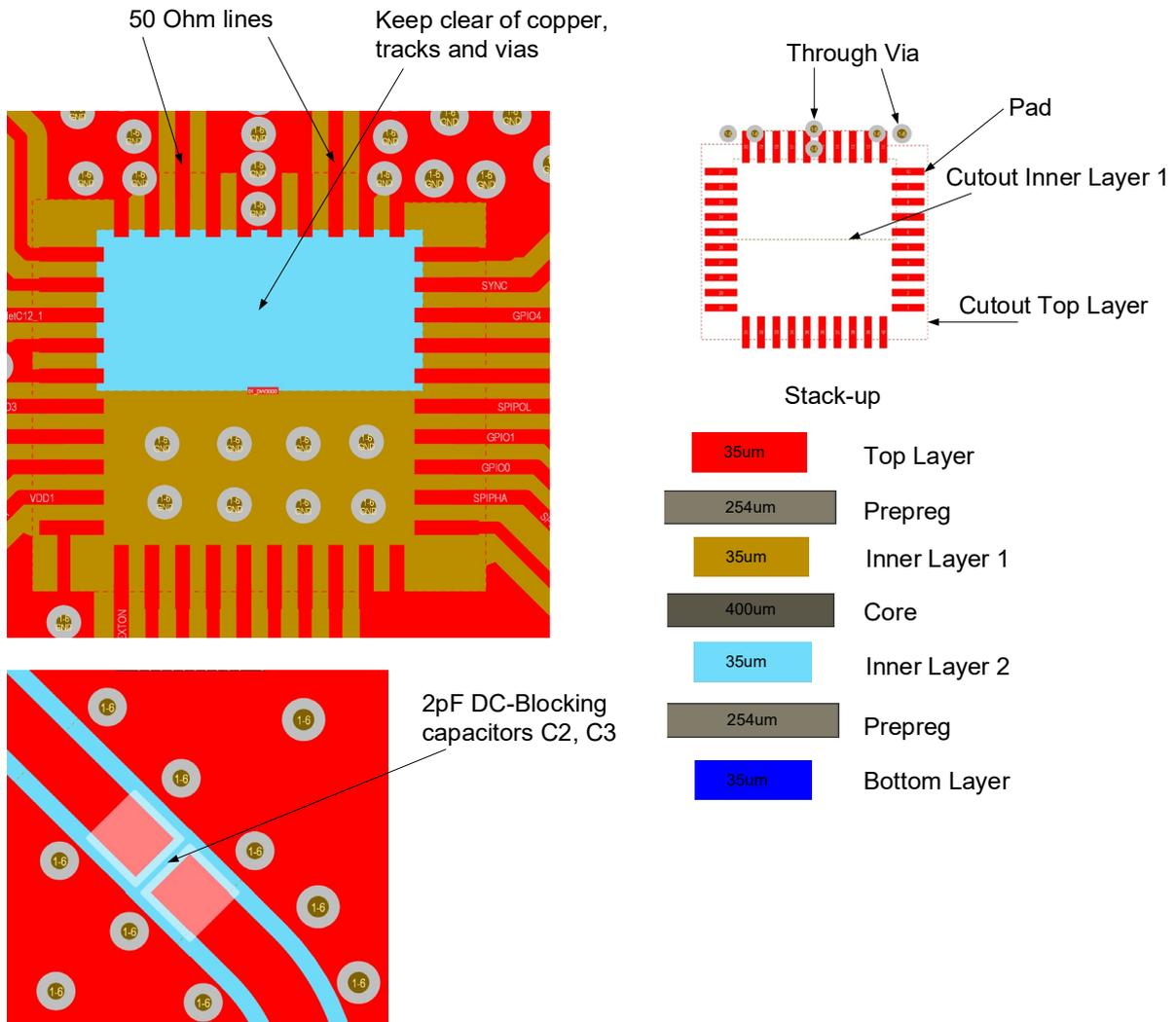
Figure 35 Recommended QFN Stack-up
