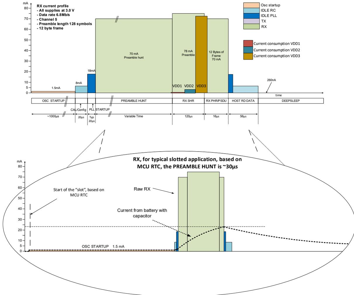
Figure 28: Current profile for receiving a frame
