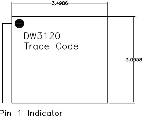
**Figure 44. New Device Package Markings (after PCN 2026)**
