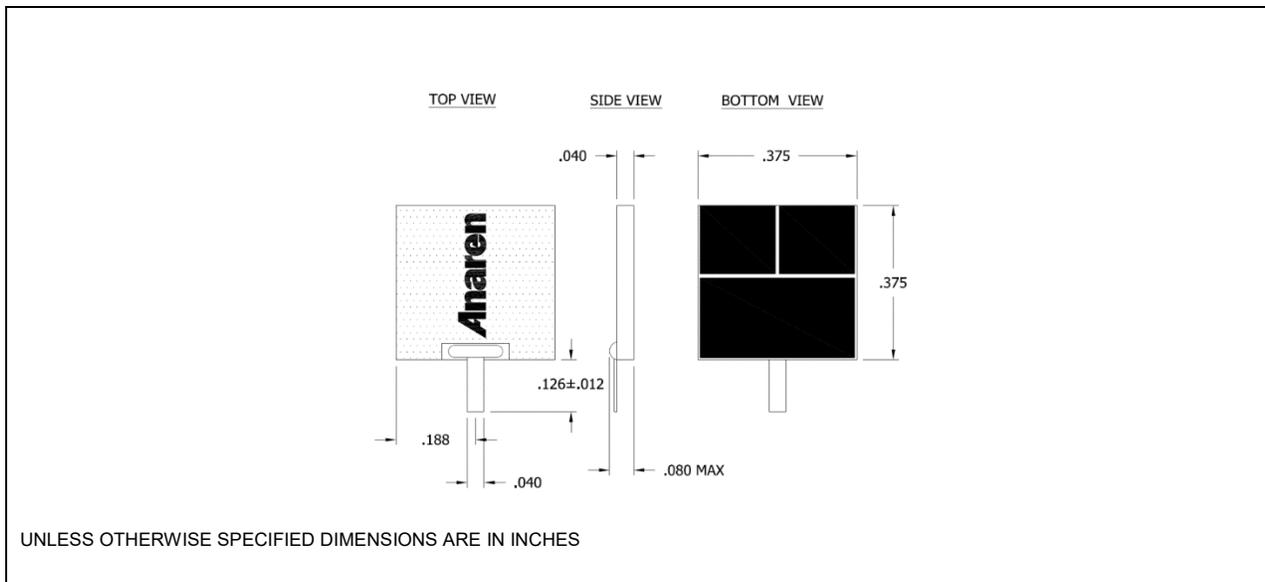
Tolerance is ±0.010", unless otherwise specified. Designed to meet or exceed applicable portions of MIL-E-5400. **All dimensions in inches.**
