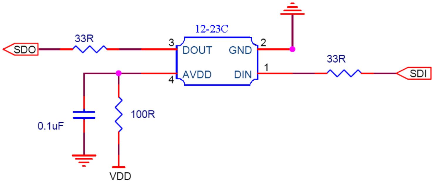
When EASV3015ICRGBA0 is set to operate on 5V power system, a 0.1uF capacitor is recommended to add between power supply and ground terminal. The capacitor is suggested to put as closer as possible to IC position. There are frequent resistors were used on different drain voltage as listed table.
