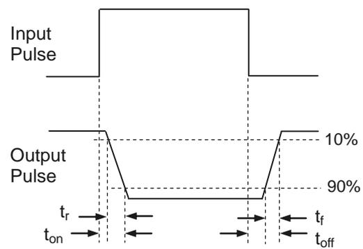
Figure 11. Switching Time Test Circuit & Waveforms
