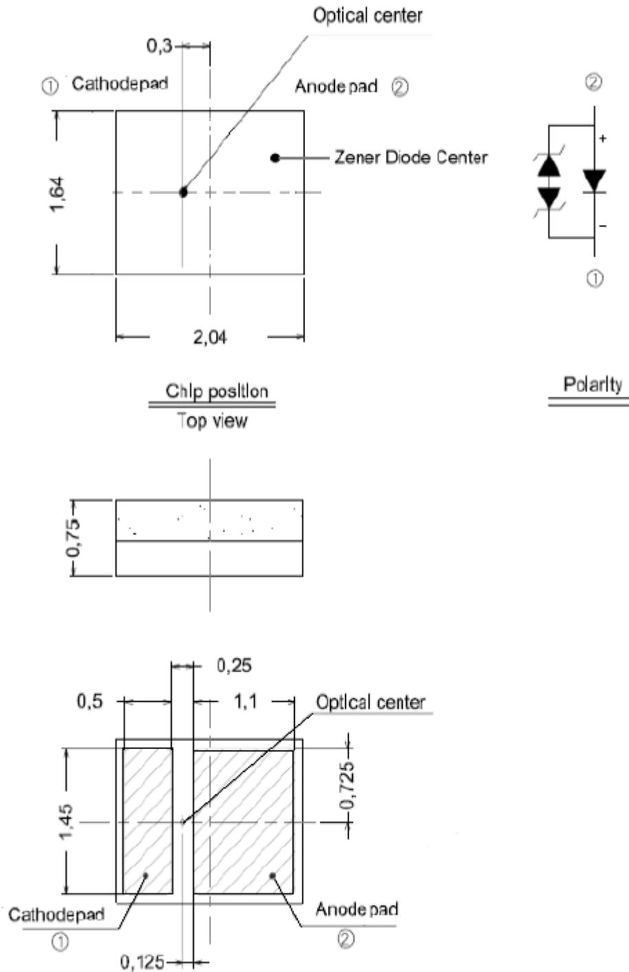
1. Dimensions are in millimeters.
