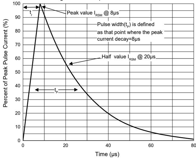
Fig. 2 - Non-Repetitive Peak Pulse Power
