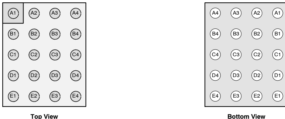
Figure 3. WLCSP-20 Pin Assignments
