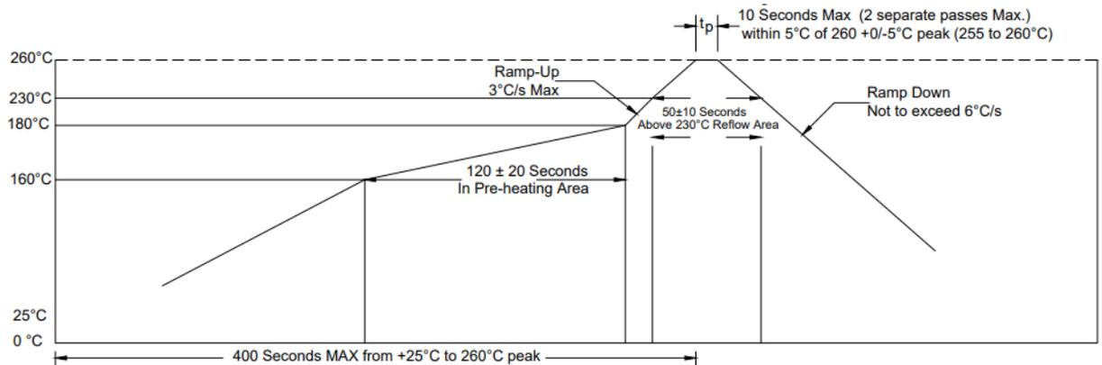
Excessive heating time at high temperature may result in deterioration of the characteristics and may break the crystal unit. For manual rework, heat the lead part at 300°C or lower for 5 seconds or less.
