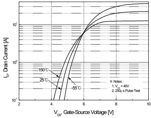
Figure 2. Transfer Characteristics
