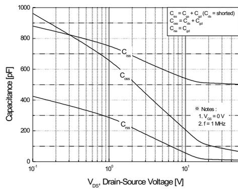
Figure 5. Capacitance Characteristics
