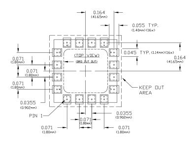
KEEP DUT AREA UNDER THE PCBDARD IS A KEEP DUT AREA, DD NDT PLACE ANY PARTS IN THIS AREA.
