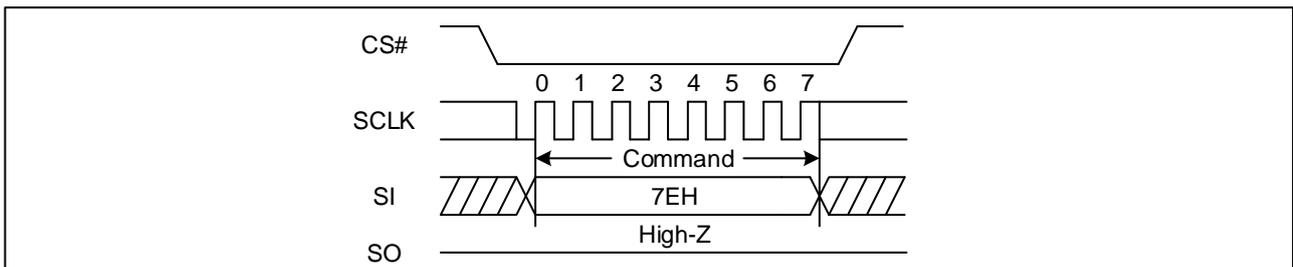
**Figure 90 Global Block/Sector Lock Sequence Diagram (QPI)**
