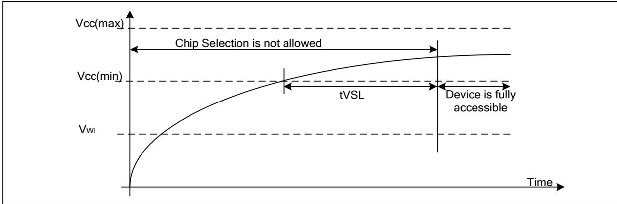
Table 17 Power-Up Timing and Write Inhibit Threshold
