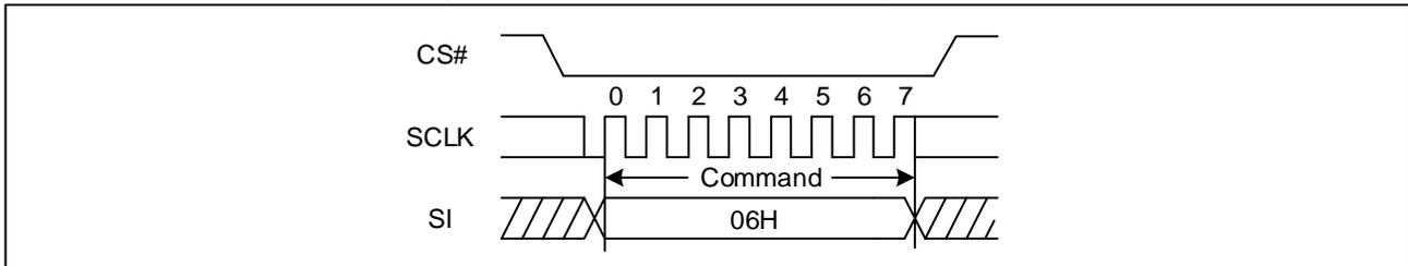
**Figure 15 Write Enable Sequence Diagram (QPI)**
