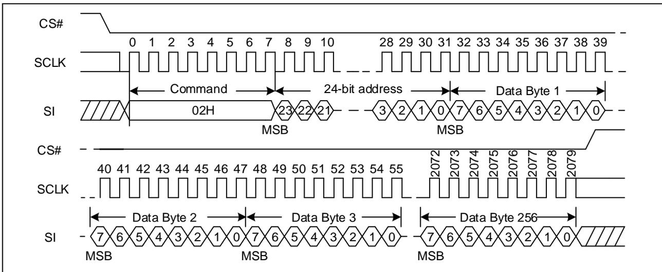
Note: The device default is in 24-bit address mode. For 4-Byte mode, the address length becomes 32-bit.
