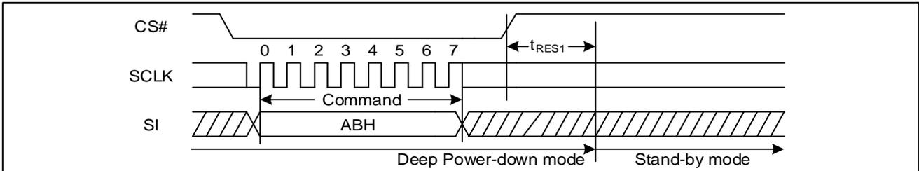
**Figure 67 Release Power-Down Sequence Diagram (QPI)**
