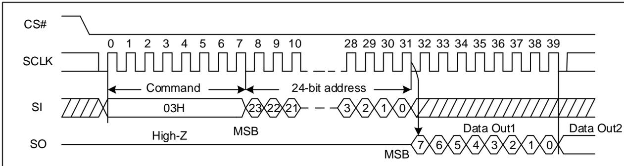
Note: The device default is in 24-bit address mode. For 4-Byte mode, the address length becomes 32-bit.
