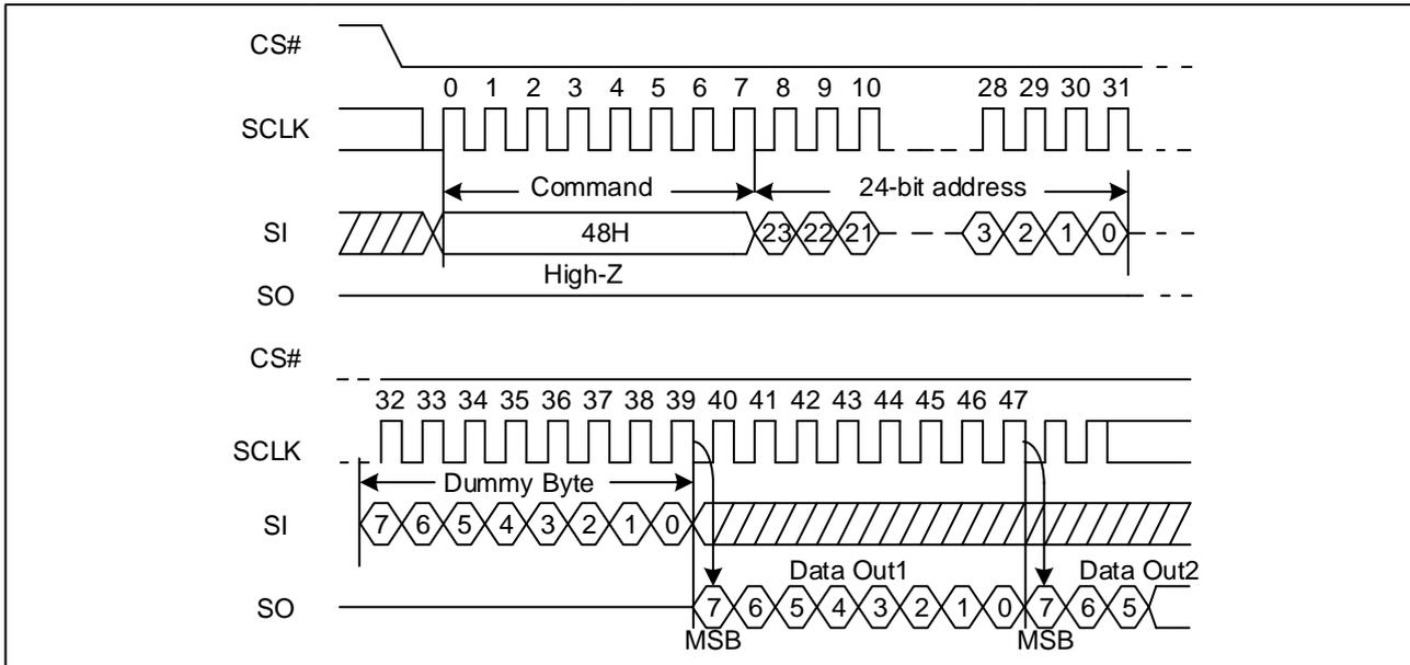
Note: The device default is in 24-bit address mode. For 4-Byte mode, the address length becomes 32-bit.
