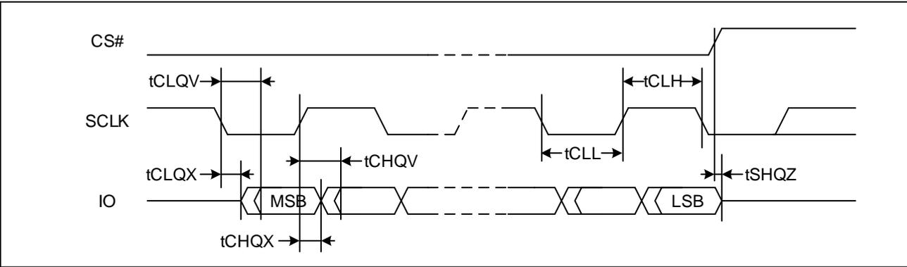
Figure 104. Resume to Suspend Timing Diagram
