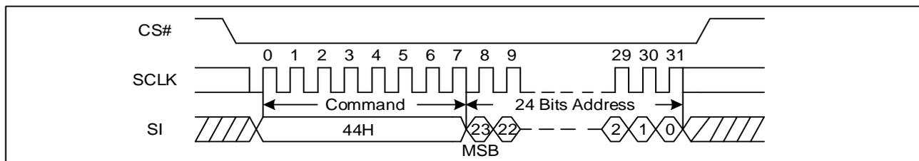
Note: The device default is in 24-bit address mode. For 4-Byte mode, the address length becomes 32-bit.
