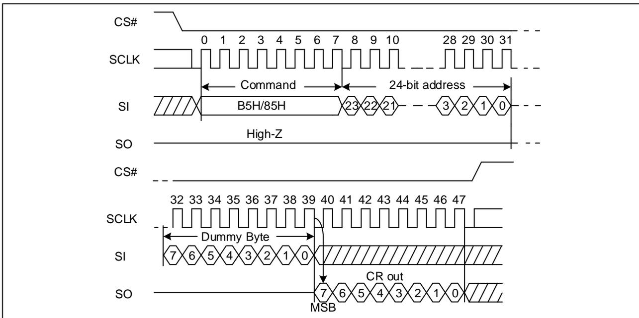
Note: The device default is in 24-bit address mode. For 4-Byte mode, the address length becomes 32-bit.
