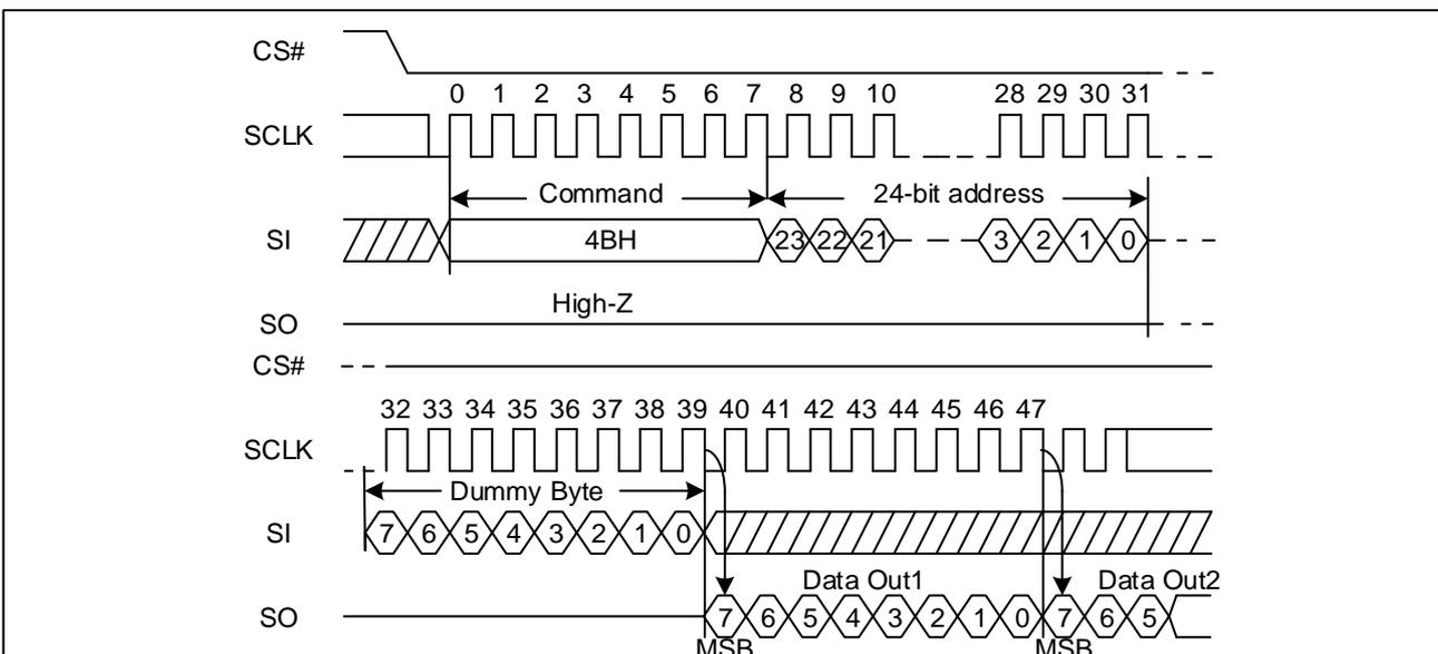
Note: The device default is in 24-bit address mode. For 4-Byte mode, the address length becomes 32-bit.
