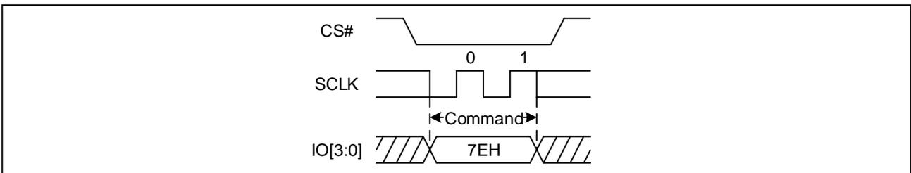
**Figure 91 Global Block/Sector Unlock Sequence Diagram (SPI)**
