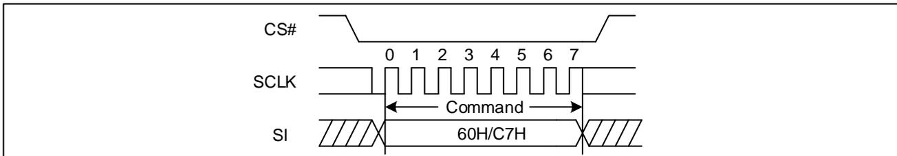
**Figure 61 Chip Erase Sequence Diagram (QPI)**
