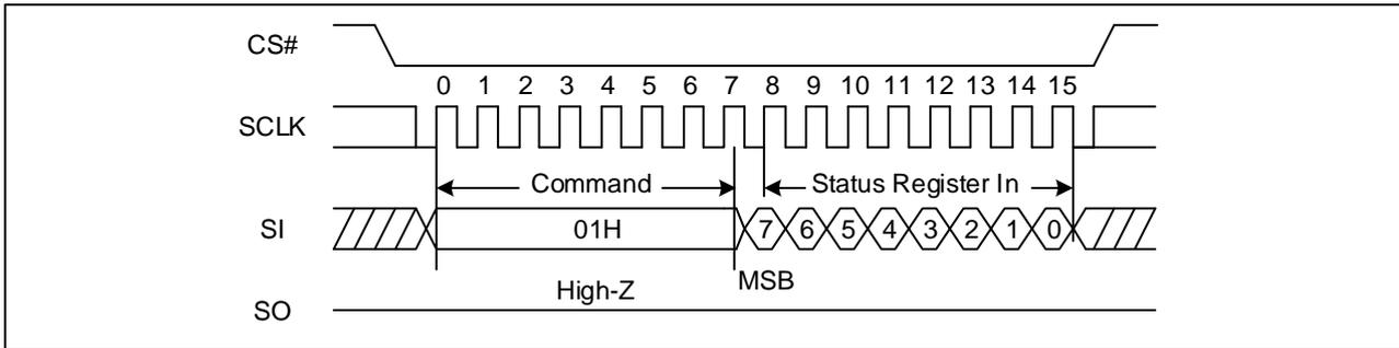
**Figure 21 Write Status Register Sequence Diagram (QPI)**
