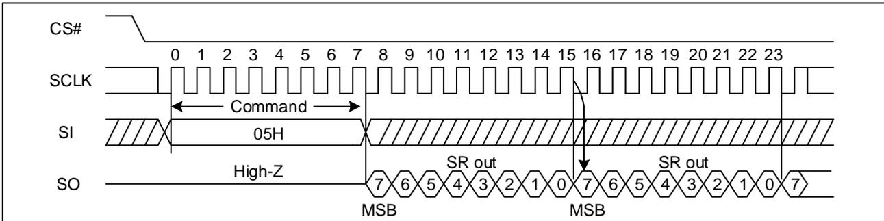
**Figure 27 Read Status Register Sequence Diagram (QPI,  $f_{SCLK} \leq 104\text{MHz}$ )**
