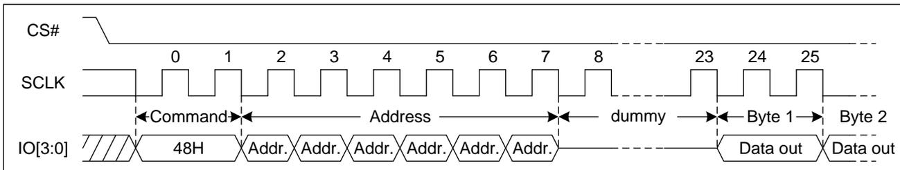
Note: The device default is in 24-bit address mode. For 4-Byte mode, the address length becomes 32-bit.
