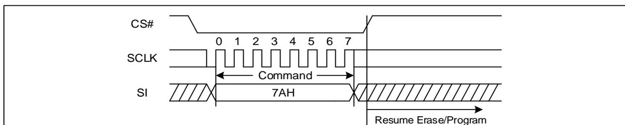
**Figure 76 Program/Erase Resume Sequence Diagram (QPI)**
