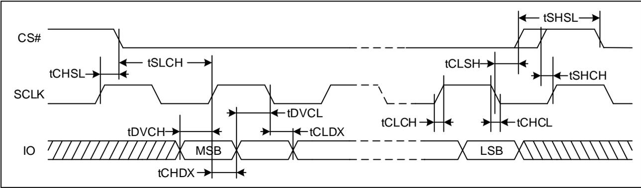
Figure 103. Serial Output Timing (DTR)
