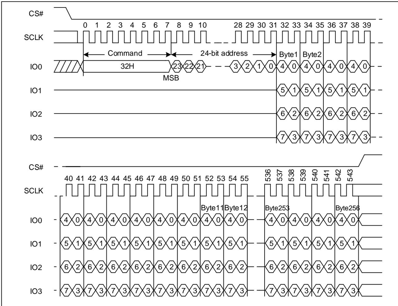
Note: The device default is in 24-bit address mode. For 4-Byte mode, the address length becomes 32-bit.
