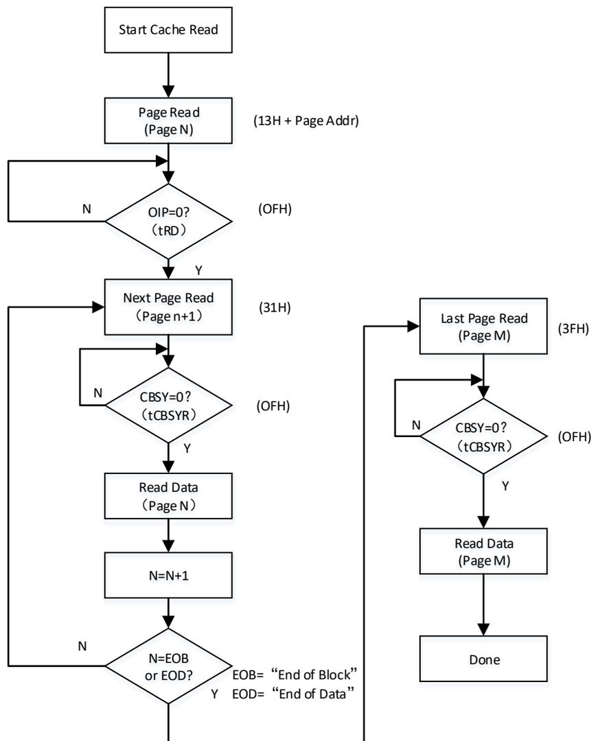
Figure 8-3. Page Read to cache Timing Diagram
