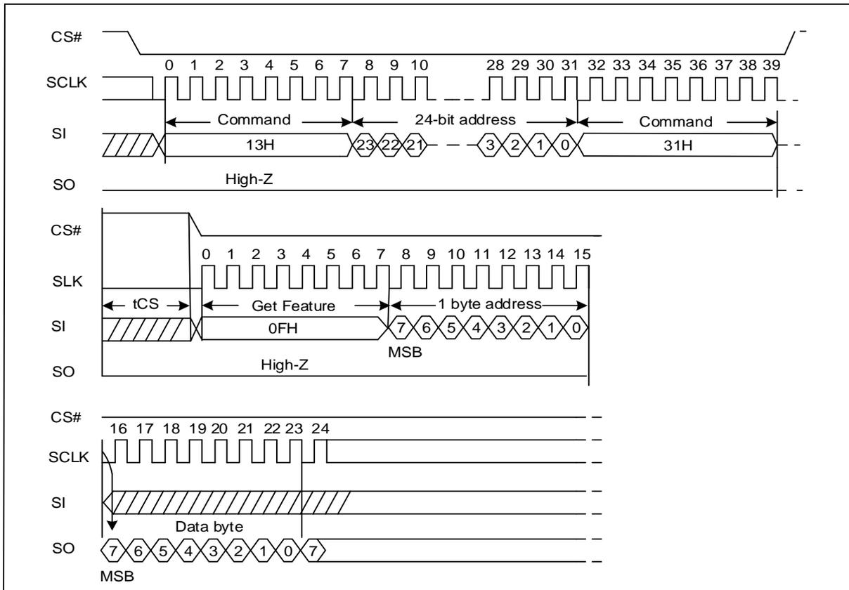
Figure 8-5. Page Read to cache Timing Diagram
