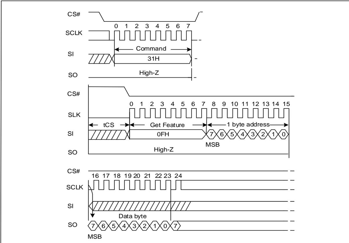
Figure 8-4. Page Read to cache Timing Diagram
