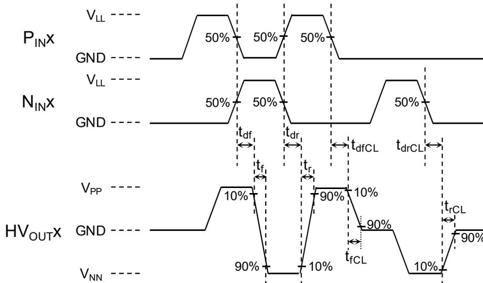
Fig.5 Propagation delay and Output rise/fall time
