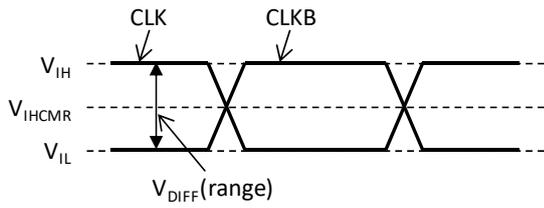
Differential input voltage peak to peak swing ( $V_{DIFF(p-p)}$ )
