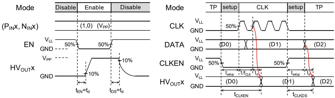
Fig.7 Output enable/disable and Clock enable/disable time
