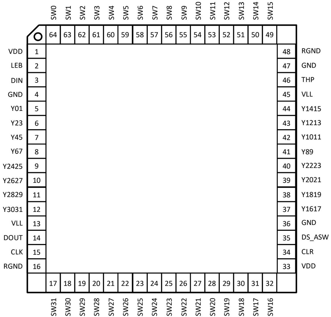
Fig.5 Pin Configuration
