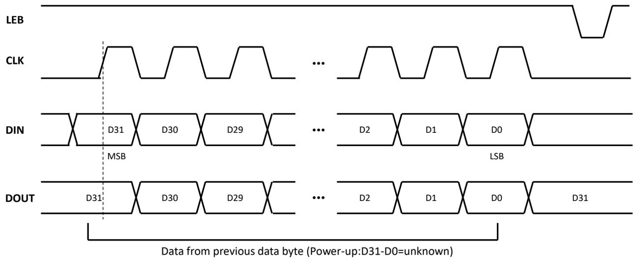
Fig.4 Latch Enable Interface Timing
