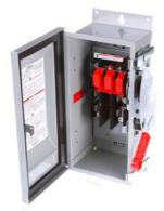
Siemens Low Voltage Circuit Protection Heavy Duty Safety Switches. Type: ENCLOSED, SAFETY SWITCH Std: UL V. Rating: 240V A. Rating: 30 A Wattage: 2W No. Of Poles: 2P F. Rating: 60Hz Action: SINGLE THROW Material: 304SS Enclosure: TYPE 12. 2-3 point mounting holes. Insulation: YES O. Cycles: 10000 O. Temperature: (-20F-120F) AMBIENT TEMPERATURE Environmental Conditions: INDUSTRIAL
