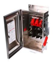
Siemens Low Voltage Circuit Protection Heavy Duty Safety Switches. Type: ENCLOSED, SAFETY SWITCH Std: UL V. Rating: 240V A. Rating: 30 A Wattage: 2W No. Of Poles: 2P F. Rating: 60Hz Action: SINGLE THROW Material: SS Enclosure: TYPE 4X. 2-3 point mounting holes. Insulation: YES O. Cycles: 10000 O. Temperature: (-20F-120F) AMBIENT TEMPERATURE Environmental Conditions: INDUSTRIAL CORROSIVE RESISTANCE
