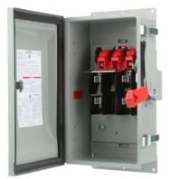
Siemens Low Voltage Circuit Protection Heavy Duty Safety Switches. Type: ENCLOSED, SAFETY SWITCH Std: UL V. Rating: 240V A. Rating: 60A Wattage: 2W No. Of Poles: 2P F. Rating: 60Hz Action: SINGLE THROW Material: 304SS Enclosure: TYPE 12. 2-3 point mounting holes. Insulation: YES O. Cycles: 10000 O. Temperature: (-20F-120F) AMBIENT TEMPERATURE Environmental Conditions: INDUSTRIAL
