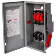
Siemens Low Voltage Circuit Protection Heavy Duty Safety Switches. Type: ENCLOSED, SAFETY SWITCH Std: CSA V. Rating: 600V A. Rating: 100A Wattage: 3W No. Of Poles: 3P F. Rating: 60Hz Action: SINGLE THROW Material: STEEL Enclosure: TYPE 1. 2-3 point mounting holes. O. Cycles: 10000 O. Temperature: (-20F-120F) AMBIENT TEMPERATURE Environmental Conditions: INDOOR
