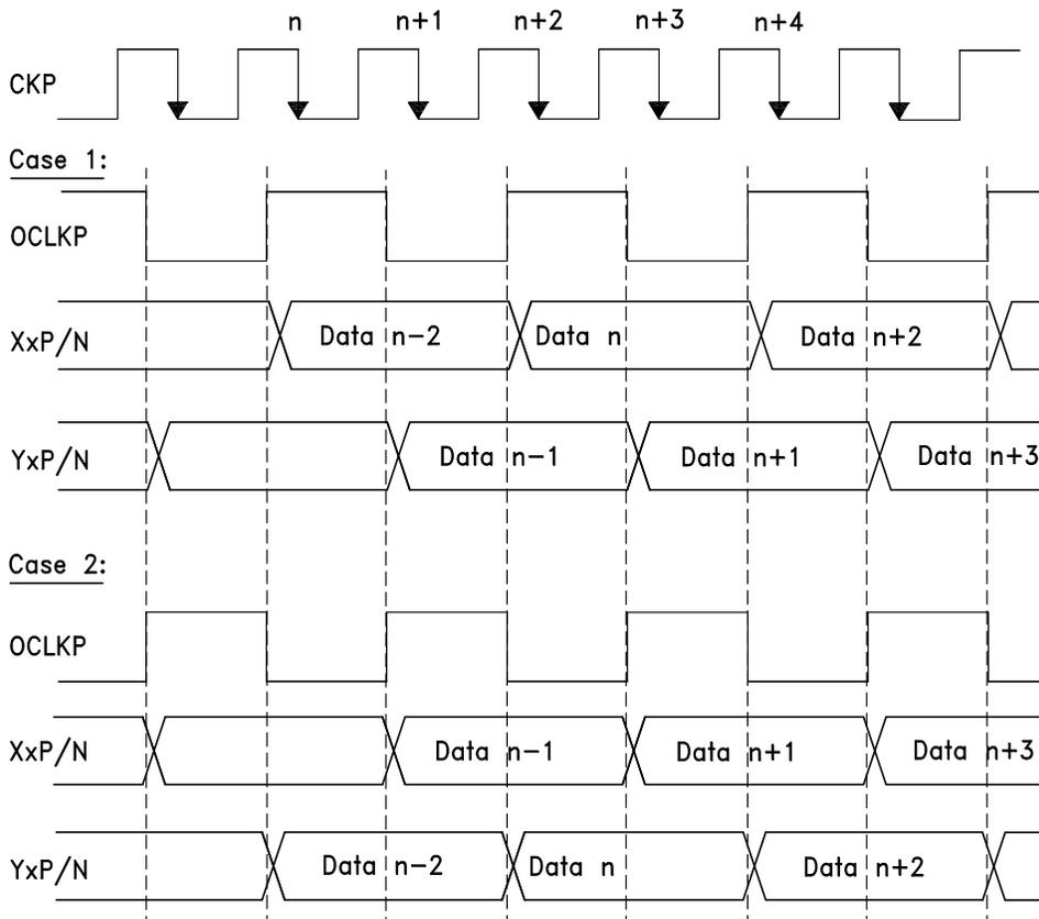
Note 1: Upon each power-up, the OCLKP signal's relationship with the CK input clock may be one of two possibilities, shown above as Case 1 and Case 2. Therefore, in reference to the OCLKP phase, the earlier data samples may be on the X or Y bus. The OCLKP's phase relationship with the X and Y data busses is fixed: the X data bus always changes with the rising edge of OCLKP and the Y bus with the falling edge.
