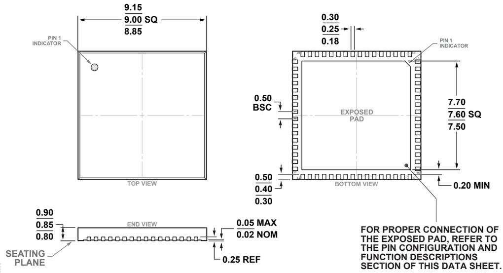
**64-Lead Lead Frame Chip Scale Package [LFCSP]
