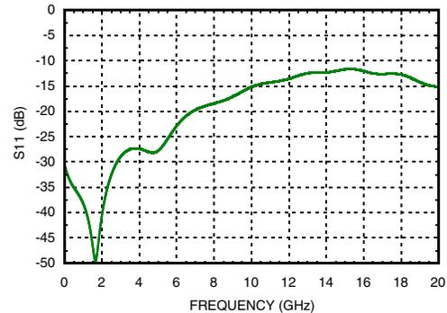
[1] This is S11 data taken from the input of the evaluation board. The gating function on the network analyzer was employed to remove the effects of the PCB and look only at the packaged part.
