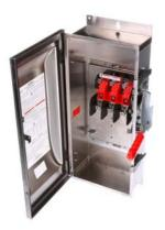
Siemens Low Voltage Circuit Protection Heavy Duty Safety Switch. 3-Pole 3-Wire Non-Fused in a type 4/4X 316 grade Stainless Steel enclosure. Rated 600VAC (30A).
