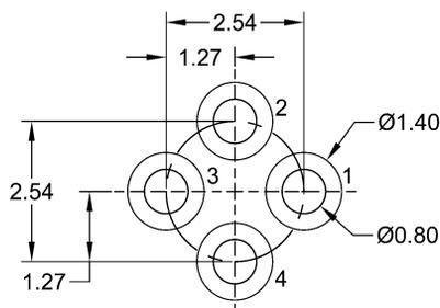
1. All linear dimensions are in millimeters.
