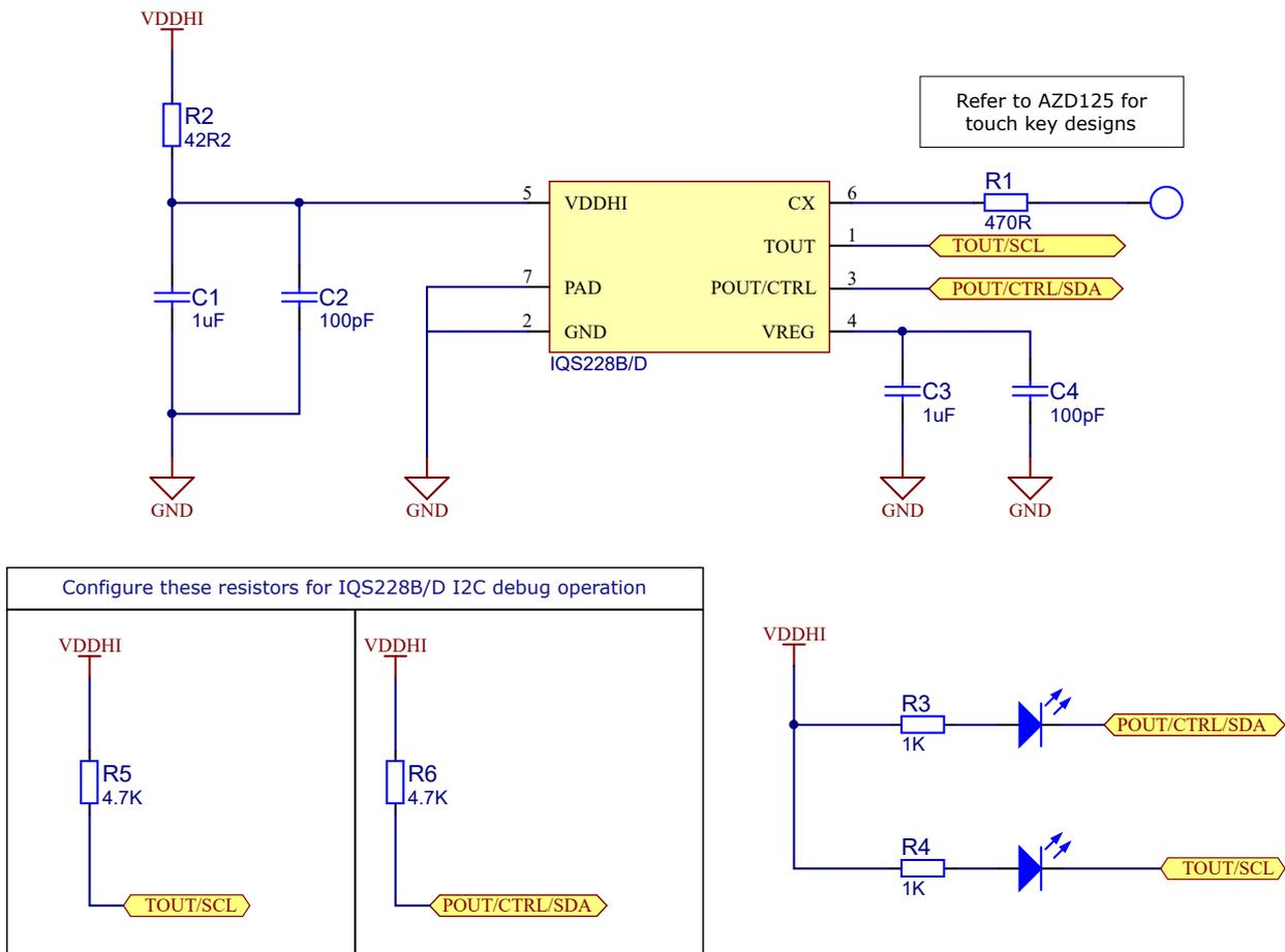
Figure 3.3: Typical application schematic of IQS228B/D. 100 pF capacitors are optional for added RF immunity. Place all decoupling capacitors (on VDDHI and VREG) as close to the IC as possible.
