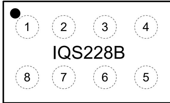
Figure 2.2: IQS228B WLCSP-8 Pin-out
