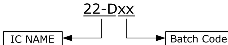
Figure 13.5: Top Marking of IQS228D
