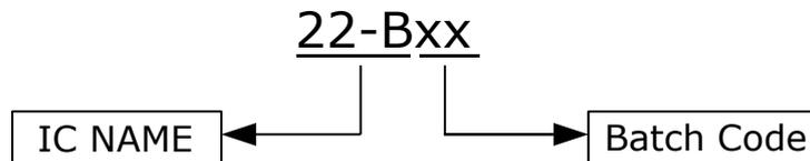
Figure 13.4: Top Marking of IQS228B
