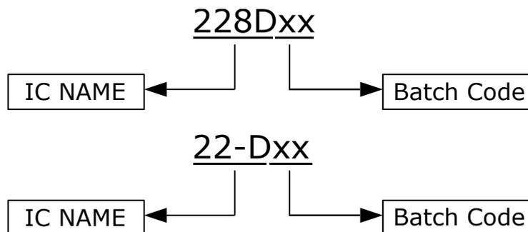
Figure 13.2: First Marking Variant of IQS228D
