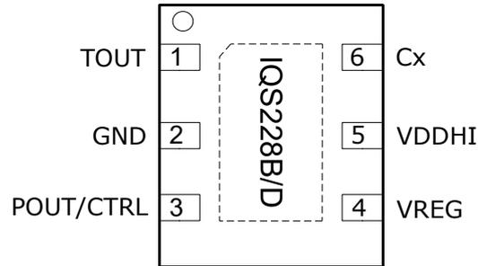
Figure 2.3: IQS228B/D DFN-6 Pin-out
