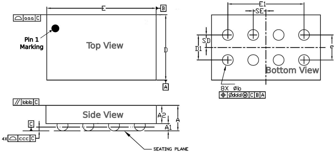
Figure 12.2: IQS228B WLCSP-8 Dimensions (in mm)
