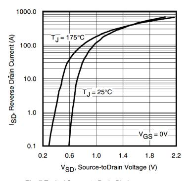
Fig. 7 Typical Source-to-Drain Diode Forward Voltage
