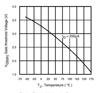
Fig 14. Threshold Voltage Vs. Temperature
