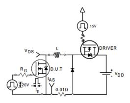
Fig. 12a. Unclamped Inductive Test Circuit
