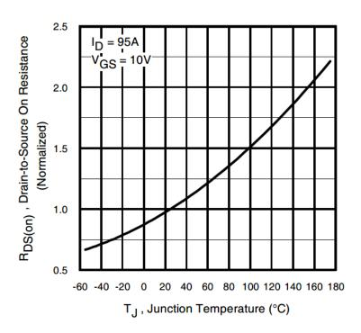
**Fig 10.** Normalized On-Resistance vs. Temperature
