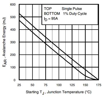
Fig 16. Maximum Avalanche Energy vs. Temperature
