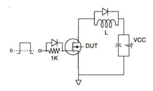
Fig 13b. Gate Charge Test Circuit
