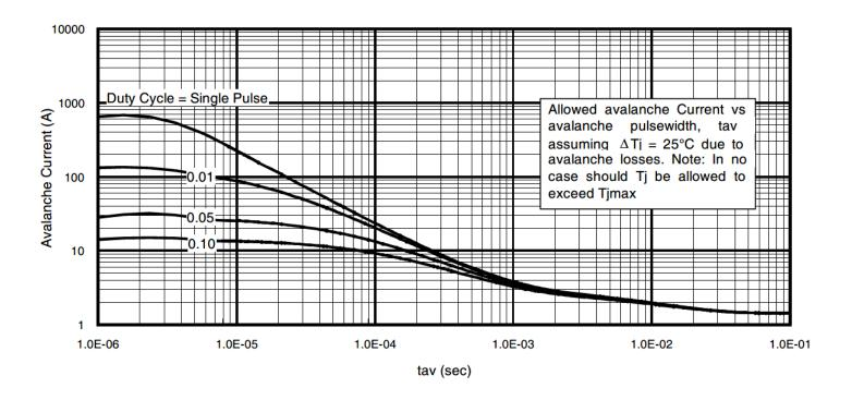
Fig. 15. Typical Avalanche Current Vs. Pulsewidth
