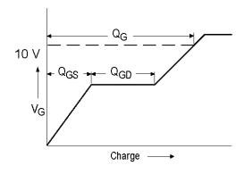
Fig 13a. Basic Gate Charge Waveform
