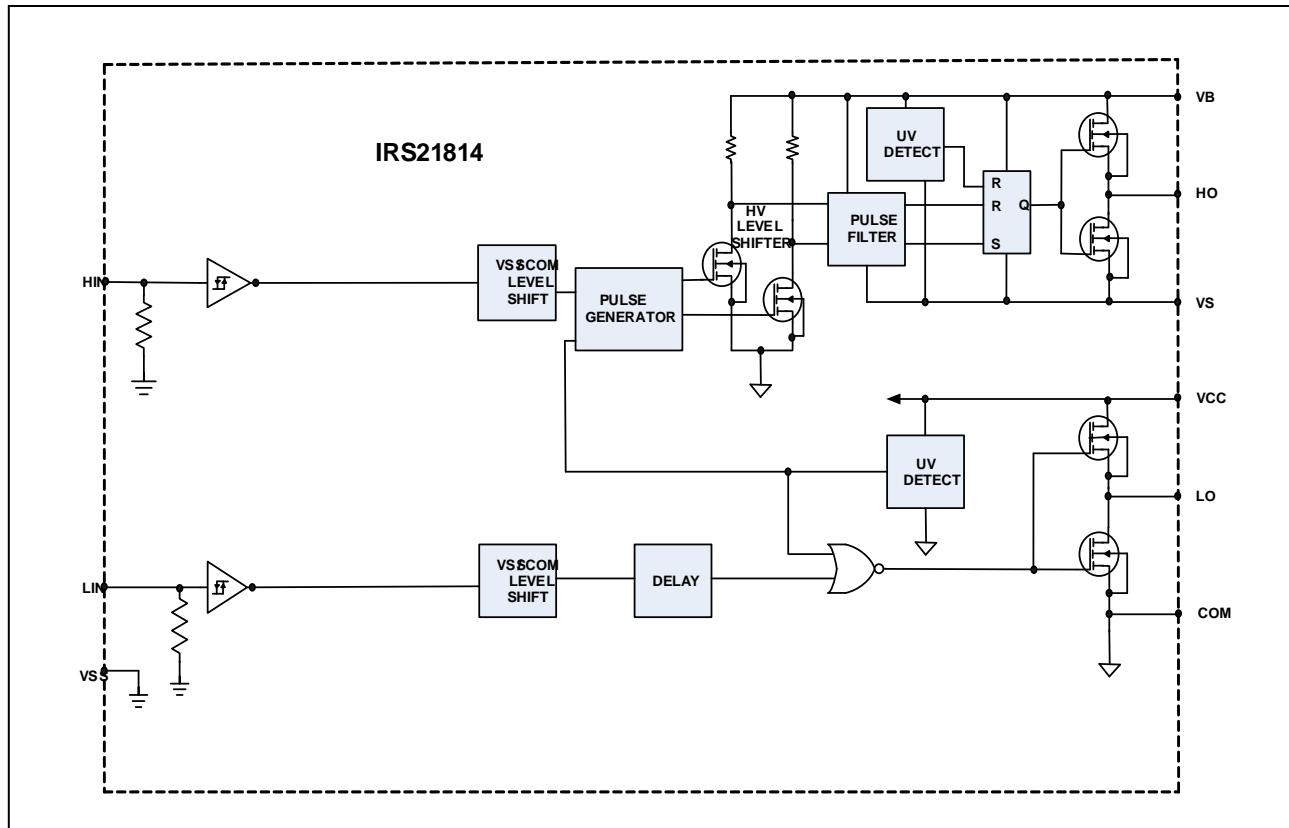
**Input/Output Pin Equivalent Circuit Diagrams: IRS21814**
