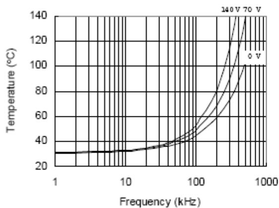
Figure 31. IRS2181S vs. Frequency (IRFB40),
