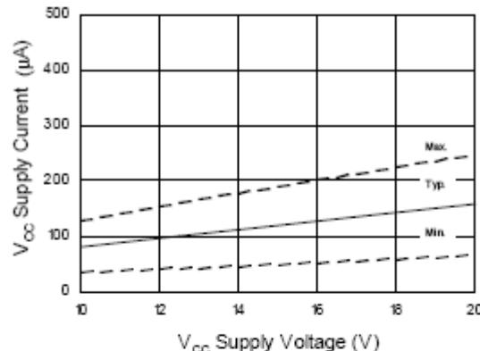
Figure 14B.  $V_{CC}$  Supply Current
