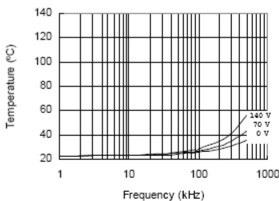
Figure 25. IRS21814 vs. Frequency (IRFBC20),
