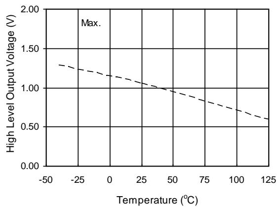
Figure 10A. High Level Output Voltage
