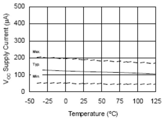
Figure 14A.  $V_{CC}$  Supply Current
