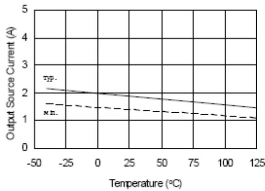
Figure 19A. Output Source Current
