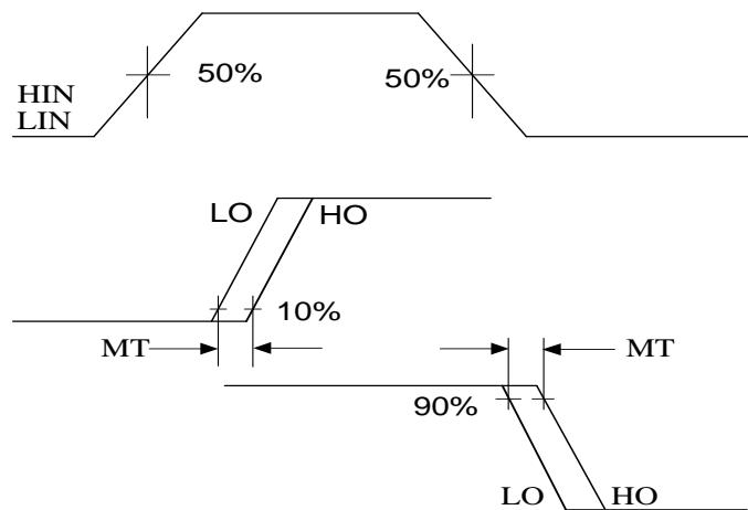
**Figure 3. Delay Matching Waveform Definitions**
