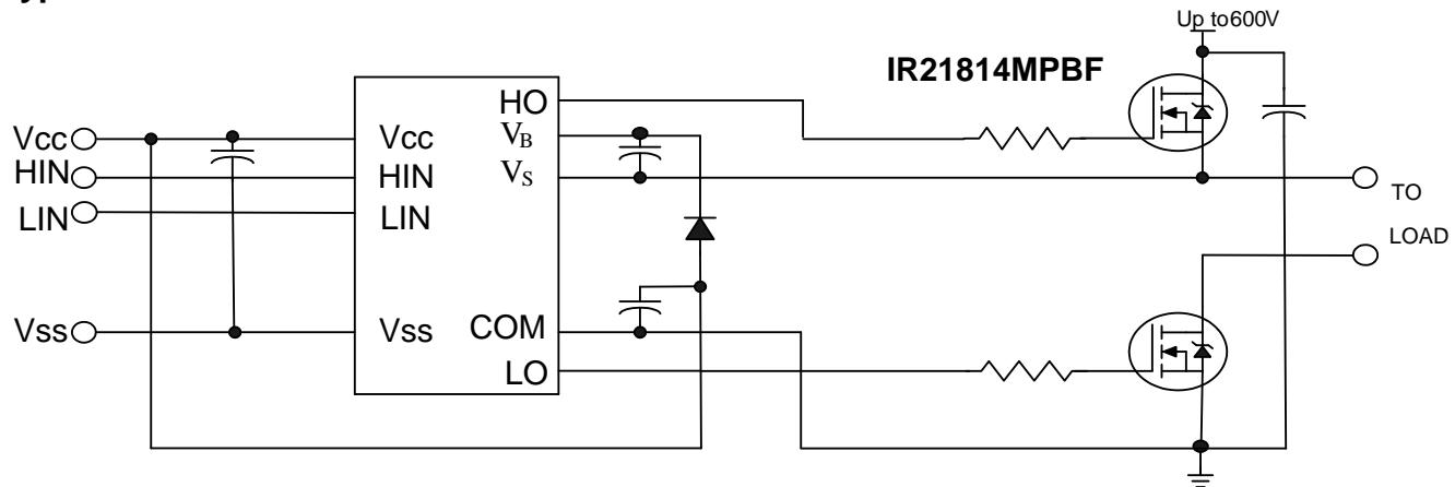
(Refer to Lead Assignments for correct pin configuration) This diagram shows electrical connections only. Please refer to our Application Notes and Design Tips for proper circuit board layout.
