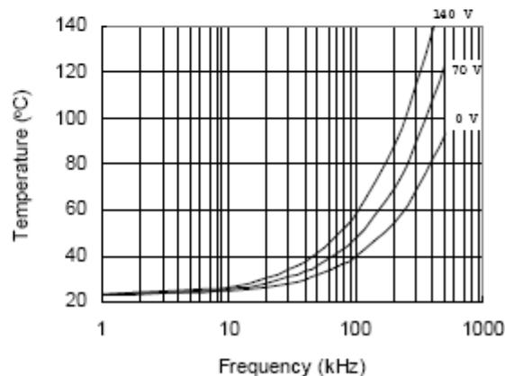
Figure 28. IRS21814 vs. Frequency (IRFPE50),
