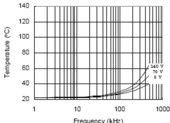
Figure 26. IRS21814 vs. Frequency (IRFBC30),
