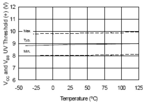
Figure 17.  $V_{CC}$  and  $V_{GS}$  Undervoltage Threshold (+)
