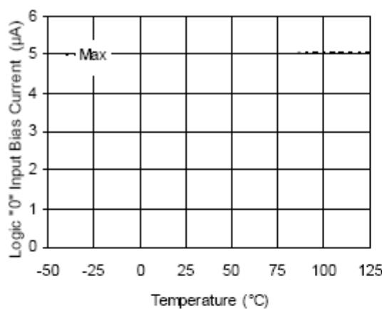
Figure 16A. Logic "0" Input Bias Current
