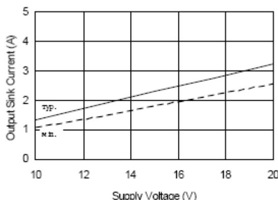
Figure 20B. Output Sink Current
