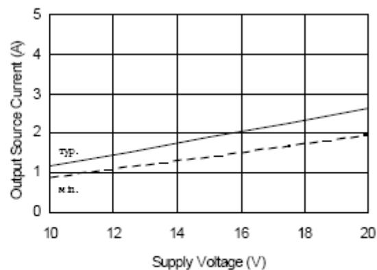
Figure 19B. Output Source Current
