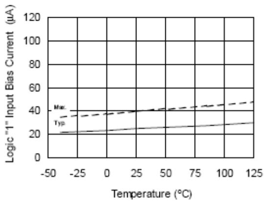
Figure 15A. Logic "1" Input Bias Current
