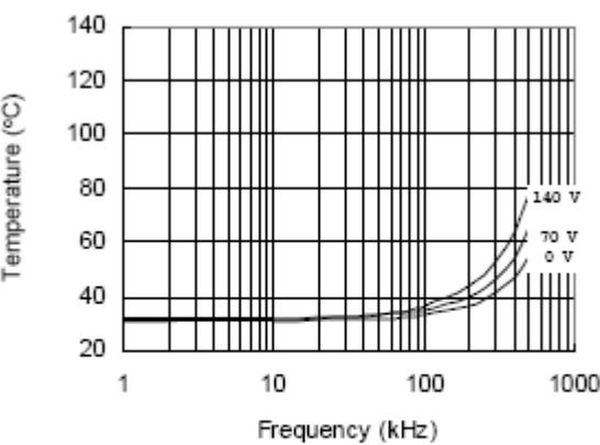
Figure 29. IRS2181S vs. Frequency (IRFBC20),
