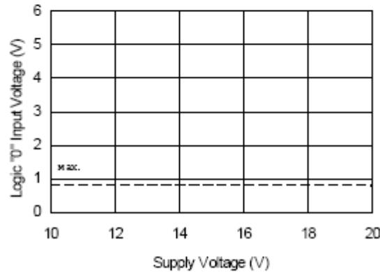
Figure 9B. Logic "0" Input Voltage
