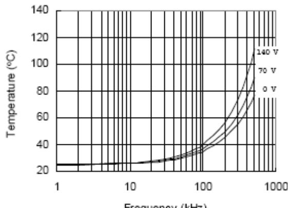
Figure 30. IRS2181S vs. Frequency (IRFBC30),
