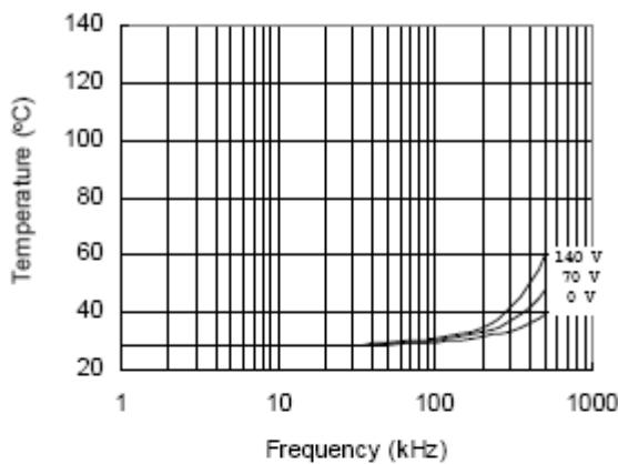
Figure 33. IRS21814S vs. Frequency (IRFB20),
