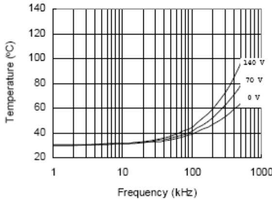
Figure 35. IRS21814S vs. Frequency (IRFB40),
