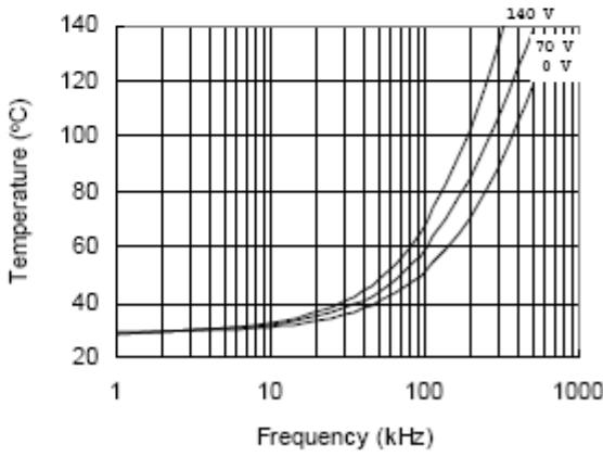
Figure 24. IRS2181 vs. Frequency (IRFPE50),
