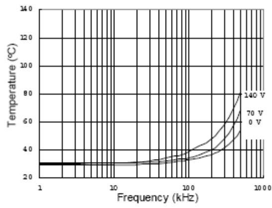
Figure 34. IRS21814S vs. Frequency (IRFBC30),
