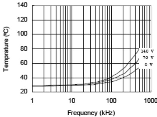
Figure 21. IRS2181 vs. Frequency (IRFBC20),
