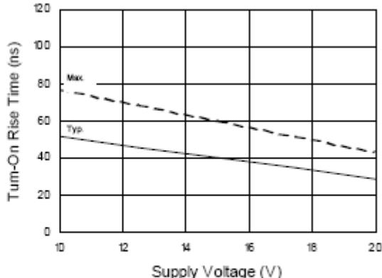
Figure 6B. Turn-On Rise Time vs. Supply Voltage
