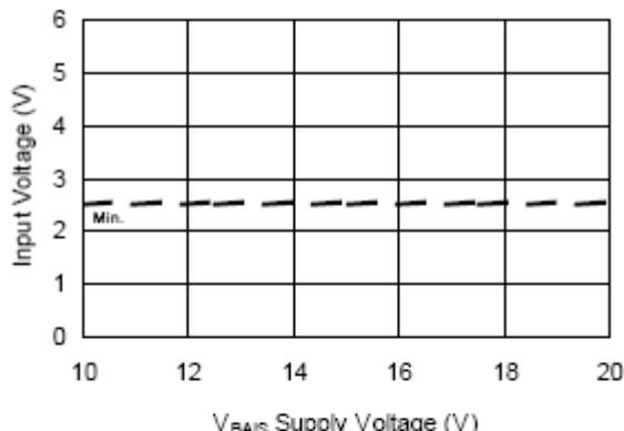
Figure 8B. Logic "1" Input voltage
