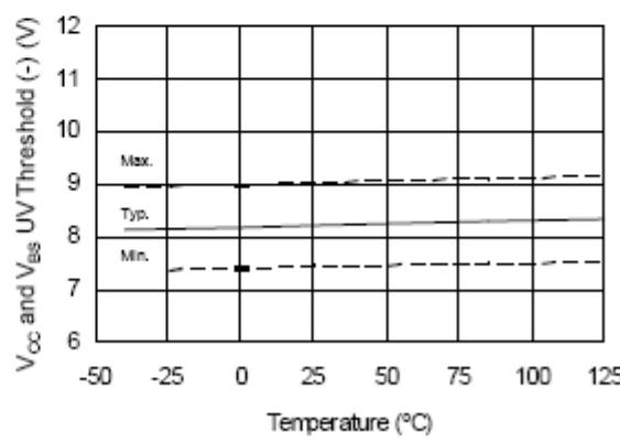
Figure 18.  $V_{CC}$  and  $V_{GS}$  Undervoltage Threshold (-)
