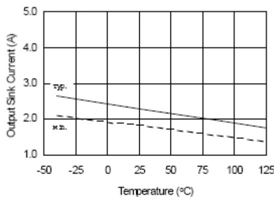
Figure 20A. Output Sink Current
