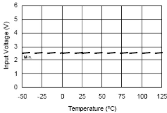
Figure 8A. Logic "1" Input Voltage
