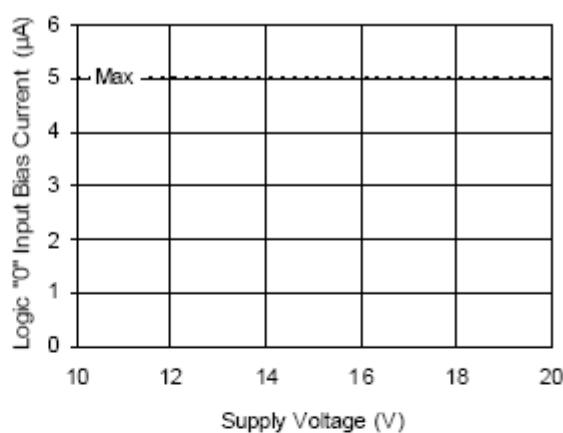
Figure 16B. Logic "0" Input Bias Current
