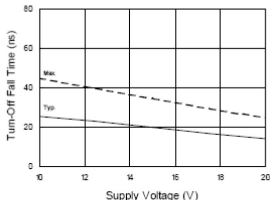
Figure 7B. Turn-Off Fall Time vs. Supply
