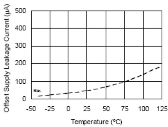
**Figure 12A. Offset Supply Leakage Current vs. Temperature**
