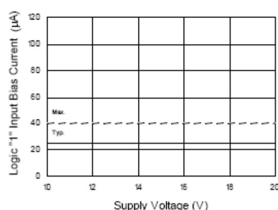
Figure 15B. Logic "1" Input Bias Current
