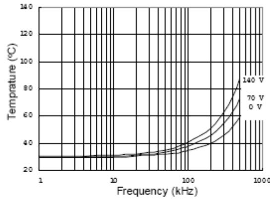
Figure 22. IRS2181 vs. Frequency (IRFBC30),
