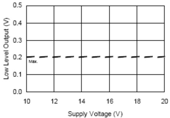
**Figure 11B. Low Level Output vs. Supply Voltage**
