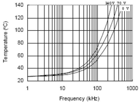
Figure 36. IRS21814S vs. Frequency (IRFPE50),
