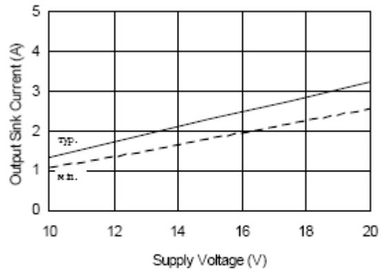
Figure 20B. Output Sink Current vs. Supply Voltage
