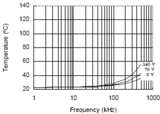
Figure 25. IRS21814 vs. Frequency (IRFBC20),
