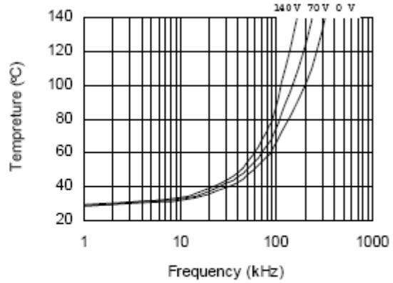
Figure 32. IRS2181S vs. Frequency (IRFPE50),
