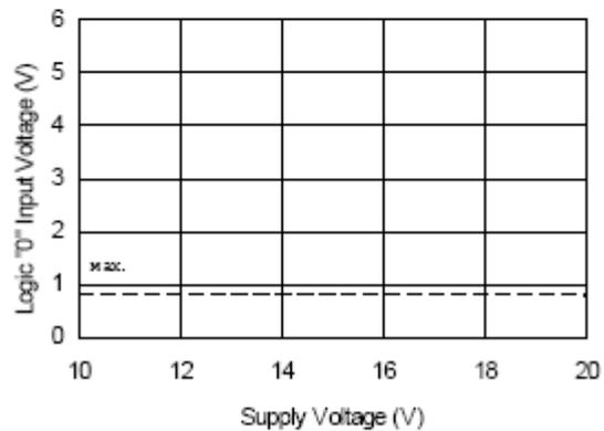
Figure 9B. Logic "0" Input Voltage vs. Supply Voltage
