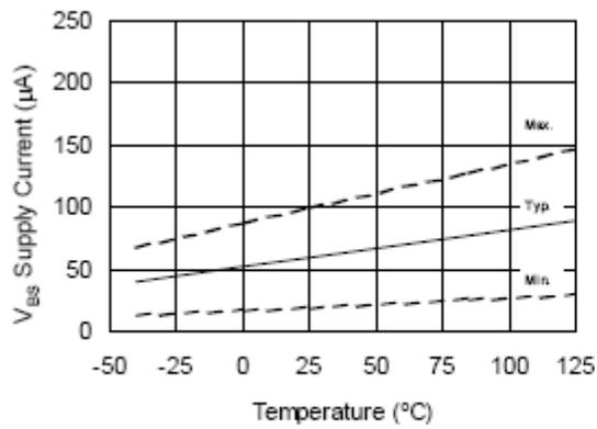
Figure 13A. V<sub>BS</sub> Supply Current vs. Temperature
