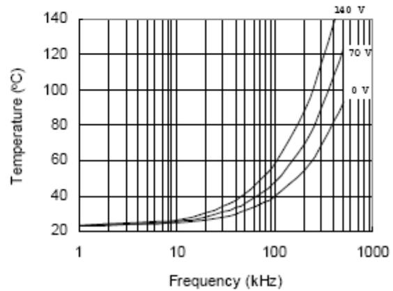
Figure 28. IRS21814 vs. Frequency (IRFPE50),
