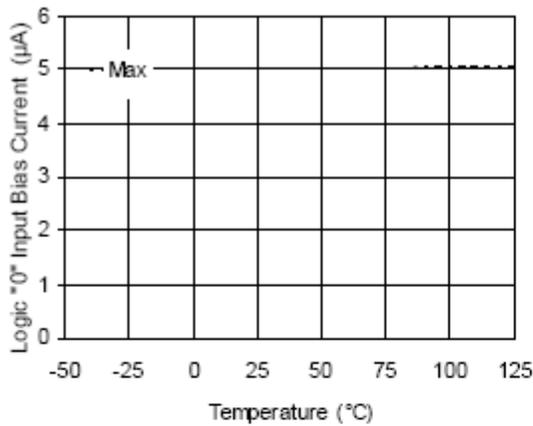
**Figure 16A. Logic "0" Input Bias Current vs. Temperature**
