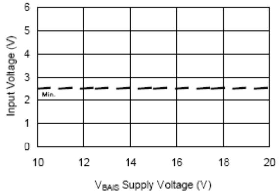
Figure 8B. Logic "1" Input Voltage vs. Supply Voltage
