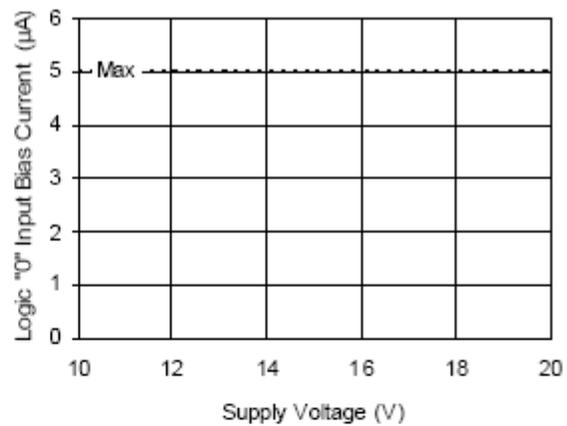
**Figure 16B. Logic "0" Input Bias Current vs. Voltage**
