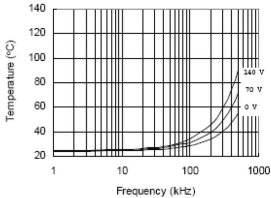
Figure 27. IRS21814 vs. Frequency (IRFBC40),
