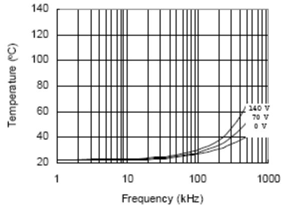
Figure 26. IRS21814 vs. Frequency (IRFBC30),
