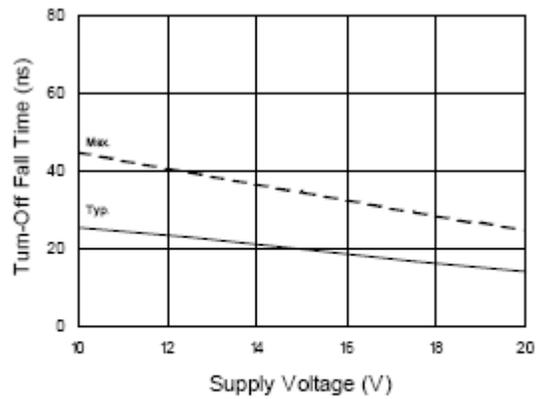
Figure 7B. Turn-Off Fall Time vs. Supply Voltage
