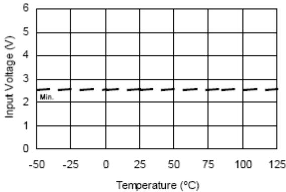
Figure 8A. Logic "1" Input Voltage vs. Temperature
