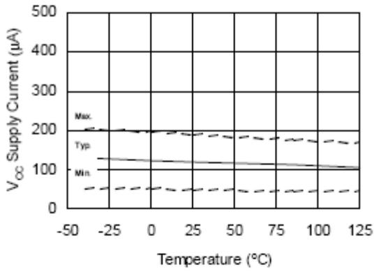
Figure 14A.  $V_{CC}$  Supply Current vs.  $V_{CC}$  Temperature
