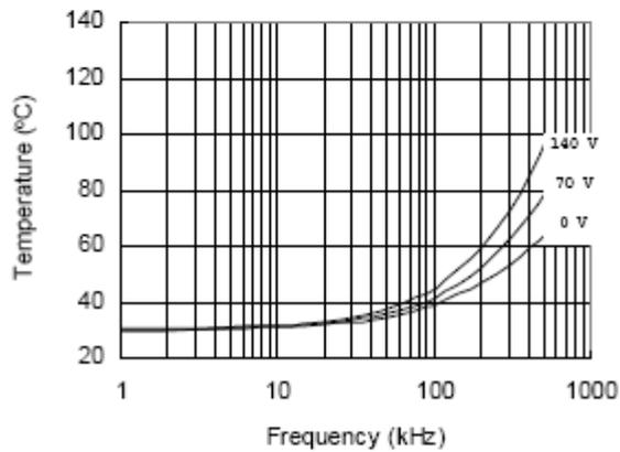
Figure 35. IRS21814S vs. Frequency (IRFBC40),
