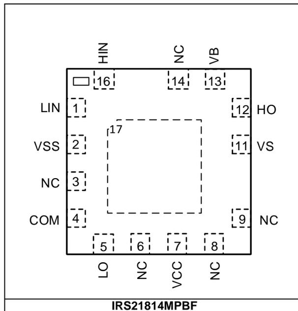
Central exposed pad (17) has to be connected to COM for better electrical performance.
