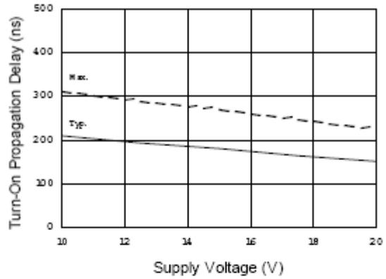
**Figure 4B. Turn-On Propagation Delay vs. Supply Voltage**
