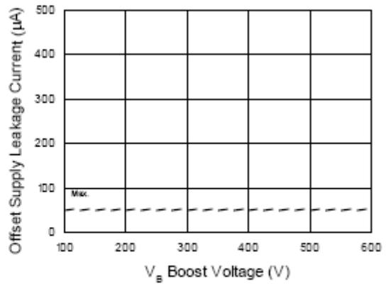
Figure 12B. Offset Supply Leakage Current vs. V<sub>B</sub> Boost Voltage
