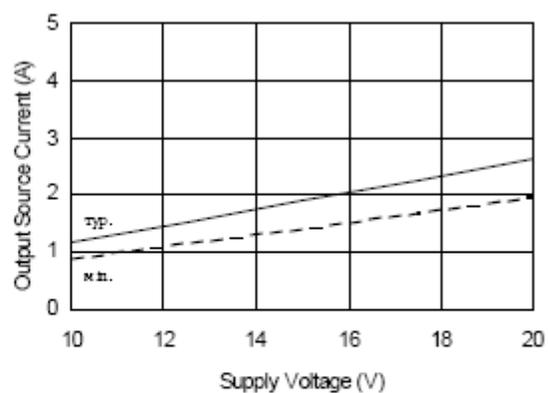
**Figure 19B. Output Source Current vs. Supply Voltage**
