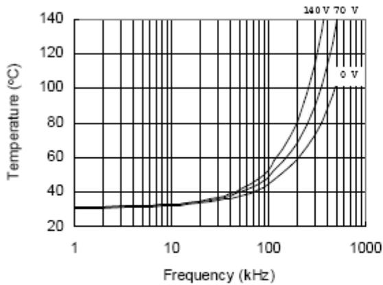
Figure 31. IRS2181S vs. Frequency (IRFBC40),
