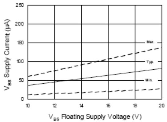
Figure 13B. V<sub>BS</sub> Supply Current vs. V<sub>BS</sub> Floating Supply Voltage
