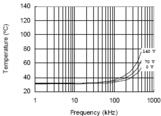
Figure 29. IRS2181S vs. Frequency (IRFBC20),
