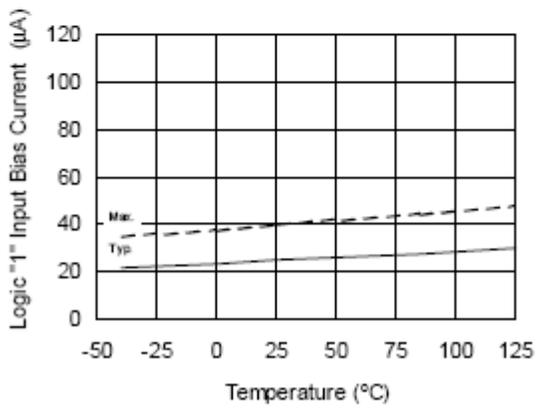
Figure 15A. Logic "1" Input Bias Current vs. Temperature
