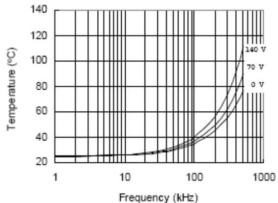
Figure 30. IRS2181S vs. Frequency (IRFBC30),
