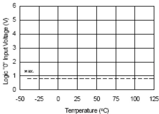
Figure 9A. Logic "0" Input Voltage vs. Temperature
