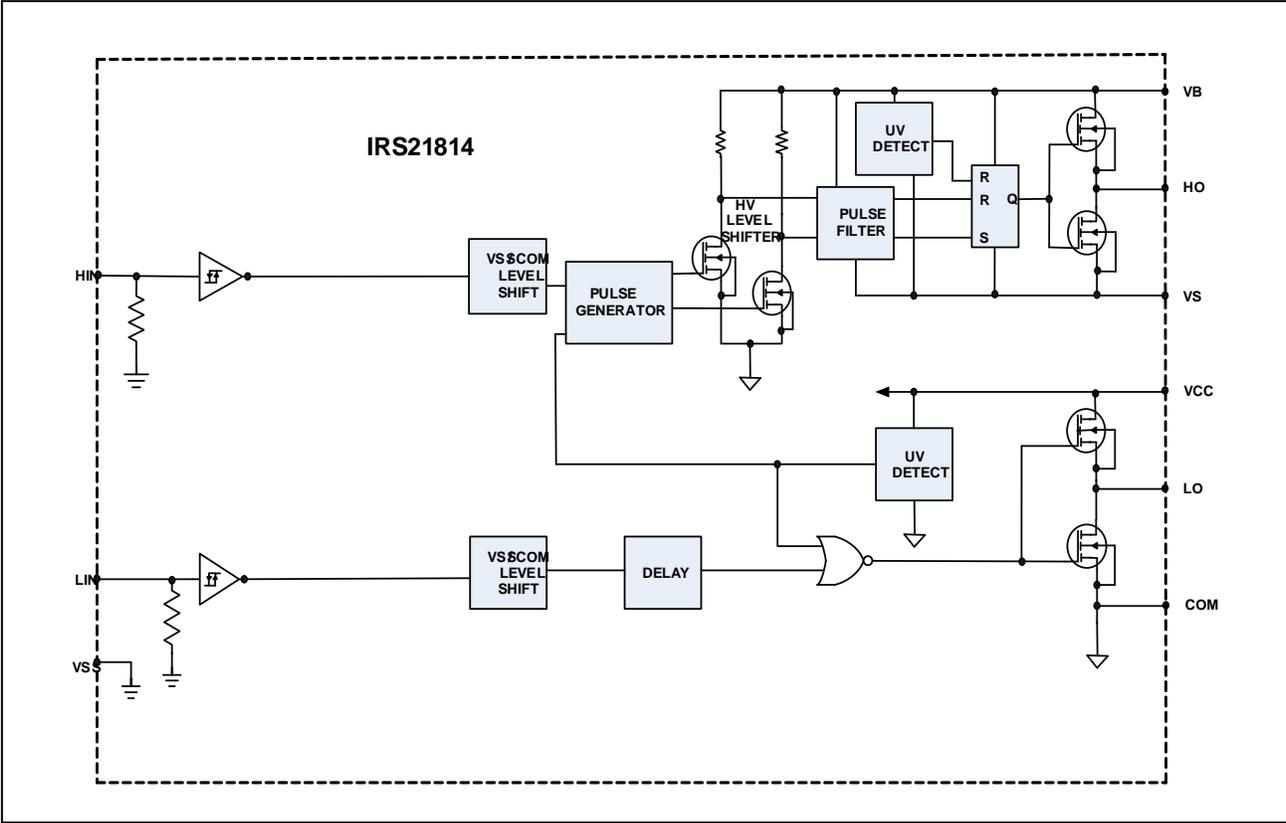
**Input/Output Pin Equivalent Circuit Diagrams: IRS21814**
