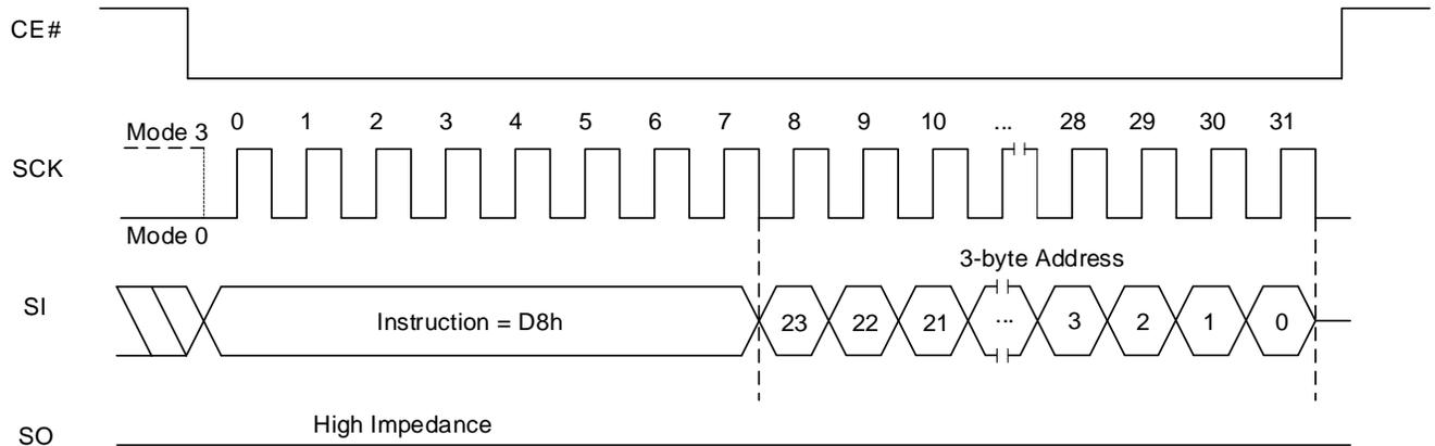
**Figure 8.17 Block Erase (64K) QPI Sequence**
