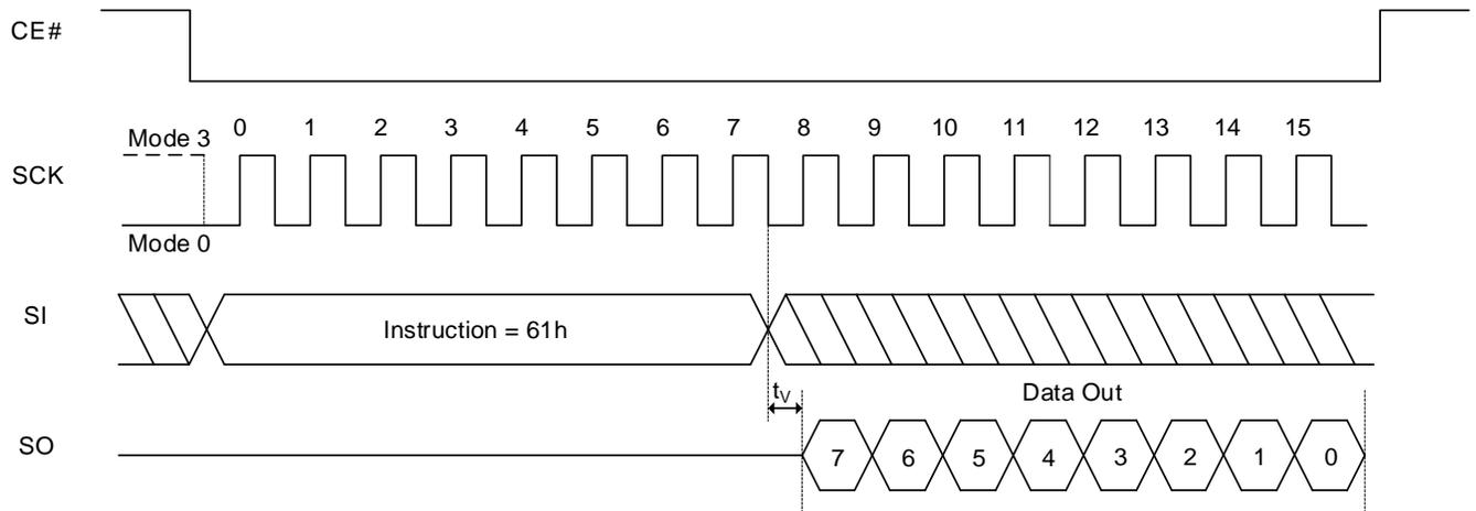
**Figure 8.45 Read Read Parameters QPI Sequence**
