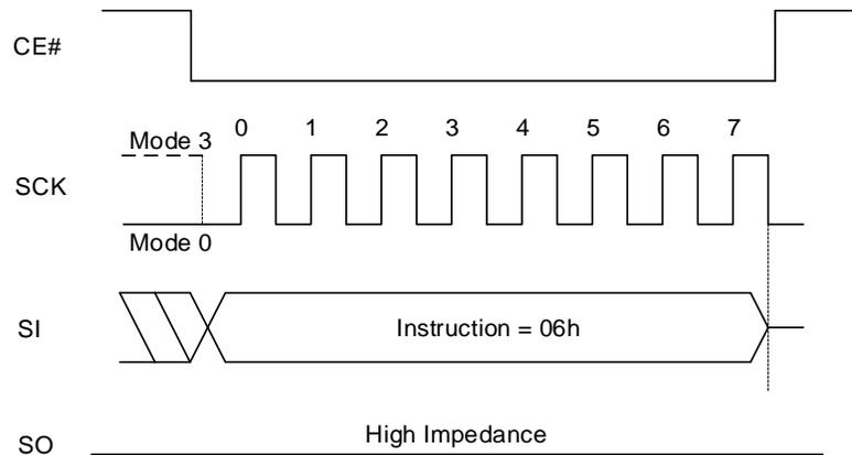
**Figure 8.23 Write Enable QPI Sequence**
