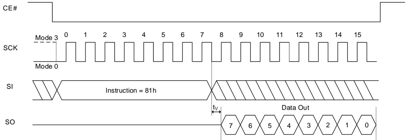
**Figure 8.47 Read Extended Read Parameters QPI Sequence**
