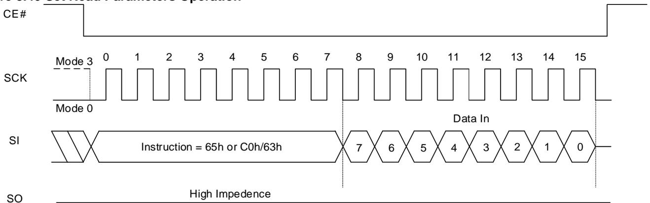
**Figure 8.41 Set Read Parameters QPI Operation**
