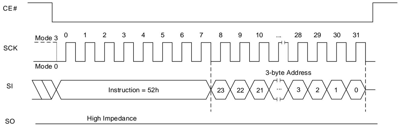
Figure 8.19 Block Erase (32K) QPI Sequence
