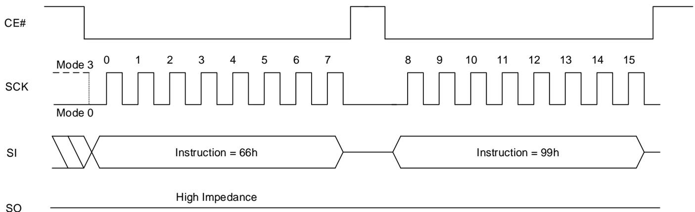
**Figure 8.57 Software Reset Enable and Software Reset QPI Sequence (RSTEN, 66h + RST, 99h)**
