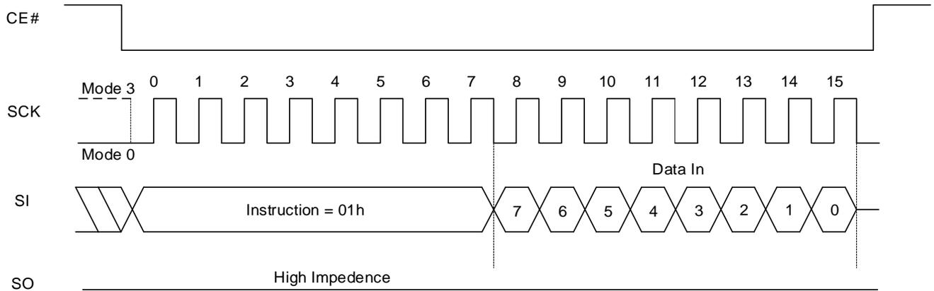
**Figure 8.29 Write Status Register QPI Sequence**
