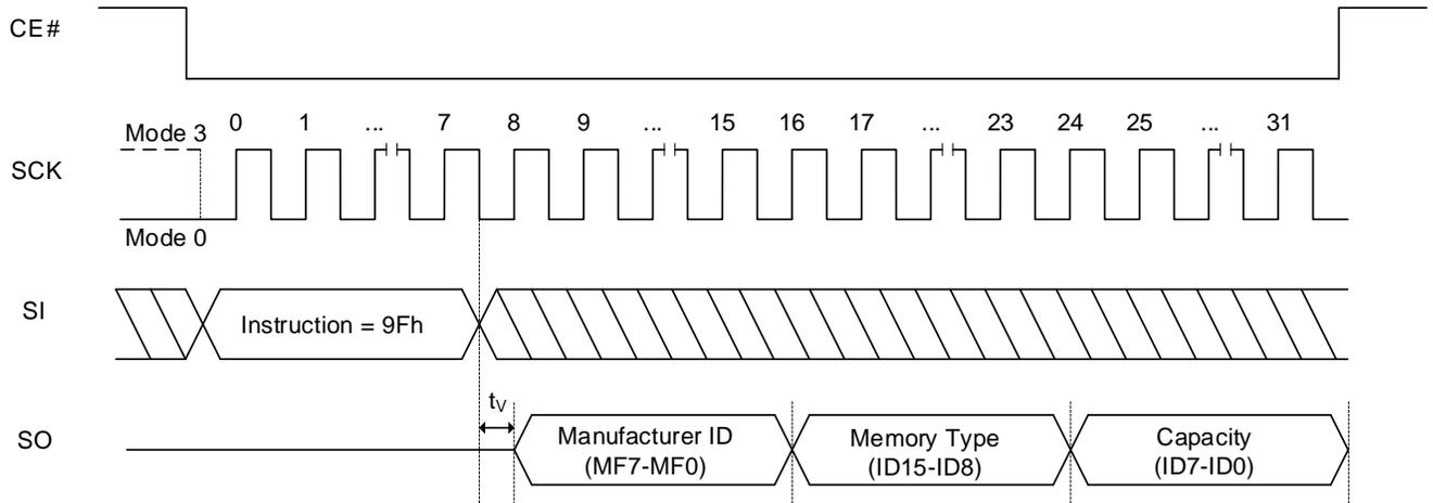
**Figure 8.51 RDJDIDQ (Read JEDEC ID in QPI Mode) Sequence**
