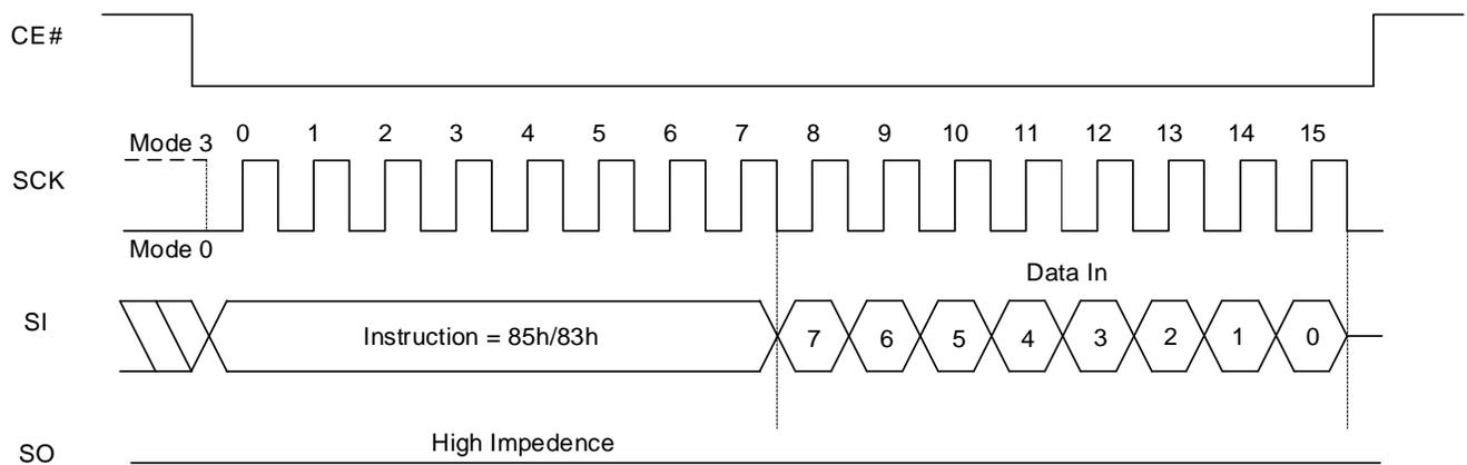
**Figure 8.43 Set Extended Read Parameters QPI Sequence**
