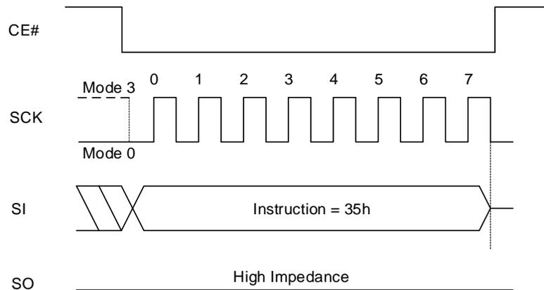
**Figure 8.35 Exit Quad Peripheral Interface (QPI) Mode Sequence**
