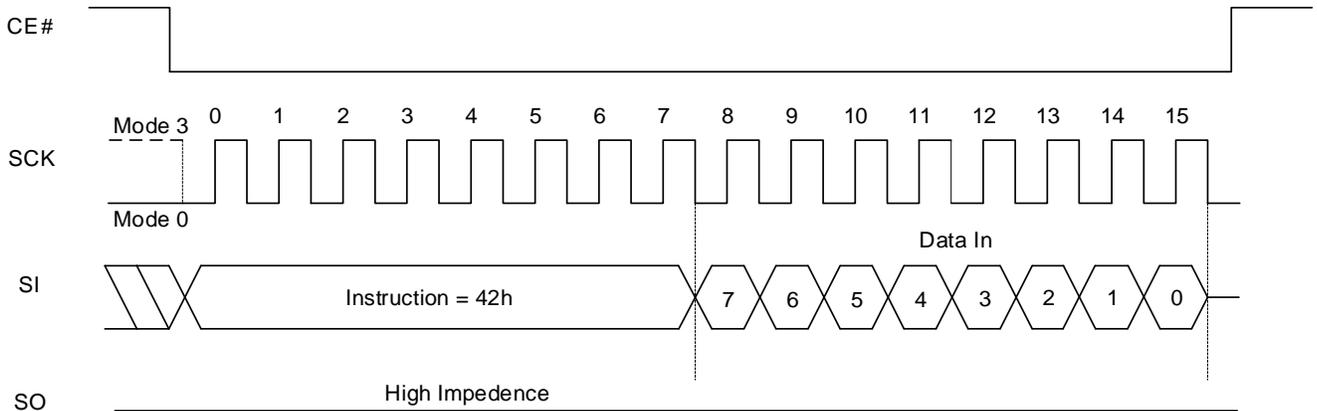
**Figure 8.33 Write Function Register QPI Sequence**
