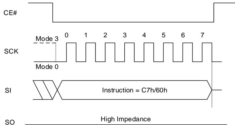
**Figure 8.21 Chip Erase QPI Sequence**
