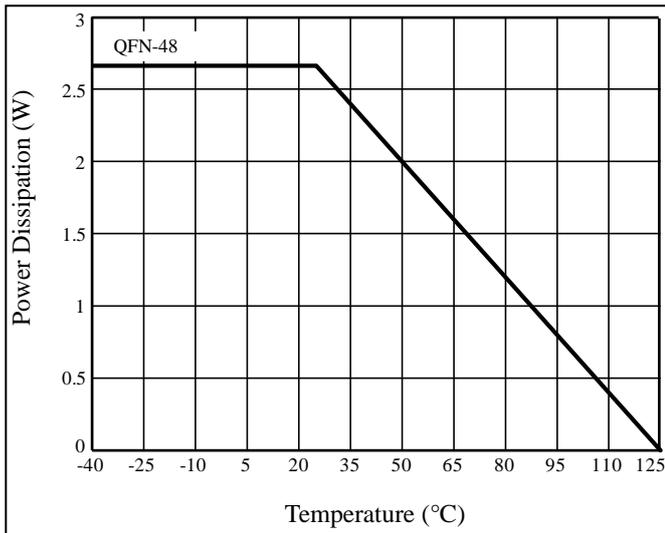
Figure 18 Dissipation Curve
