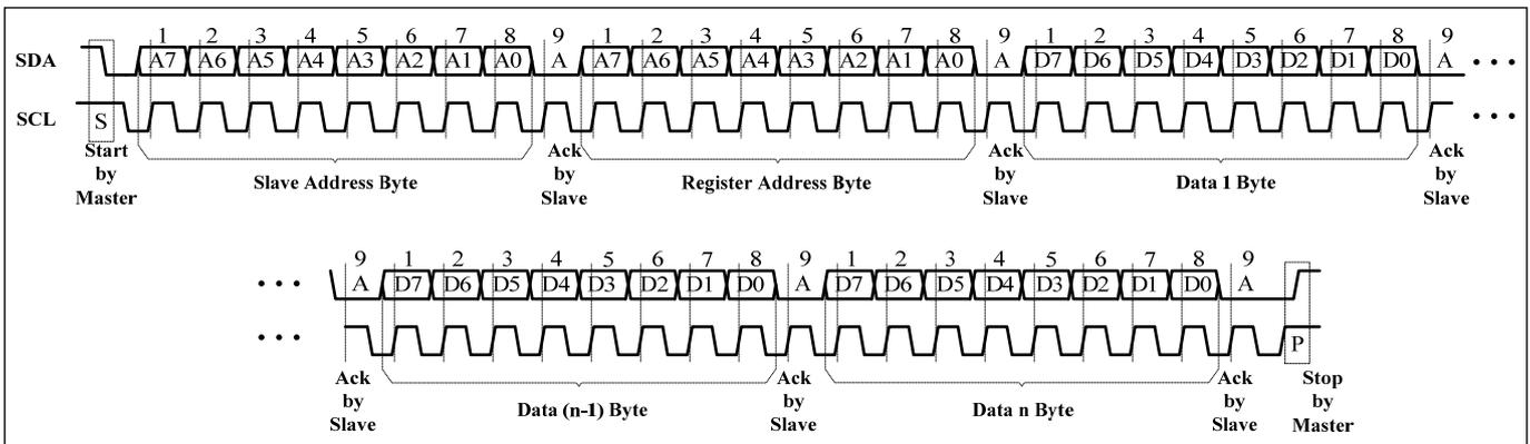
Figure 7 Writing to IS31FL3733A (Automatic Address Increment)
