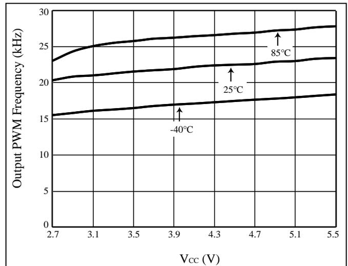
Figure 19  $V_{CC}$  vs. CSx PWM Frequency
