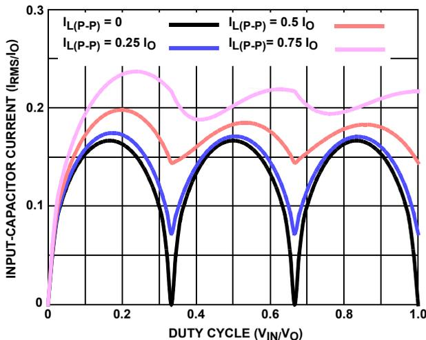
FIGURE 27. NORMALIZED INPUT-CAPACITOR RMS CURRENT FOR 3-PHASE CONVERTER
