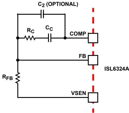
**FIGURE 23. COMPENSATION CONFIGURATION FOR LOAD-LINE REGULATED ISL6324A CIRCUIT**
