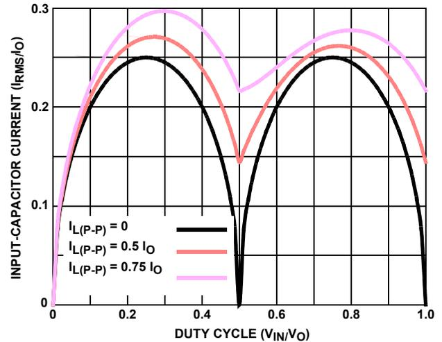
FIGURE 28. NORMALIZED INPUT-CAPACITOR RMS CURRENT FOR 2-PHASE CONVERTER
