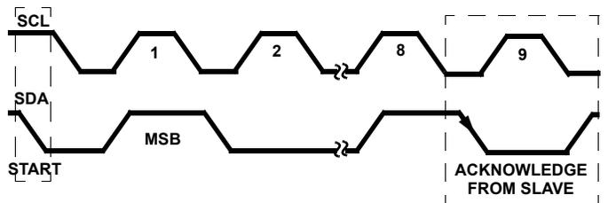
FIGURE 17. ACKNOWLEDGE ON THE I<sup>2</sup>C BUS
