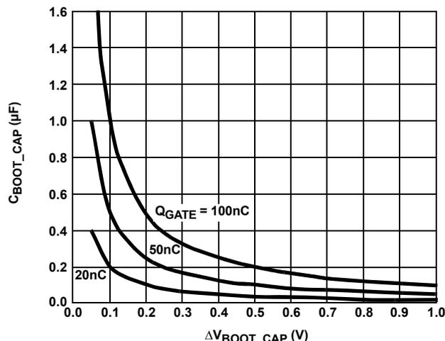
FIGURE 18. BOOTSTRAP CAPACITANCE vs BOOT RIPPLE VOLTAGE
