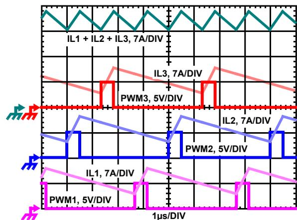
FIGURE 1. PWM AND INDUCTOR-CURRENT WAVEFORMS FOR 3-PHASE CONVERTER
