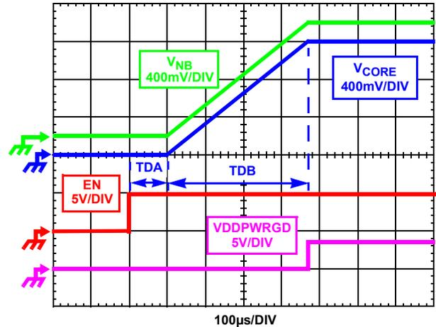
FIGURE 11. SOFT-START WAVEFORMS
