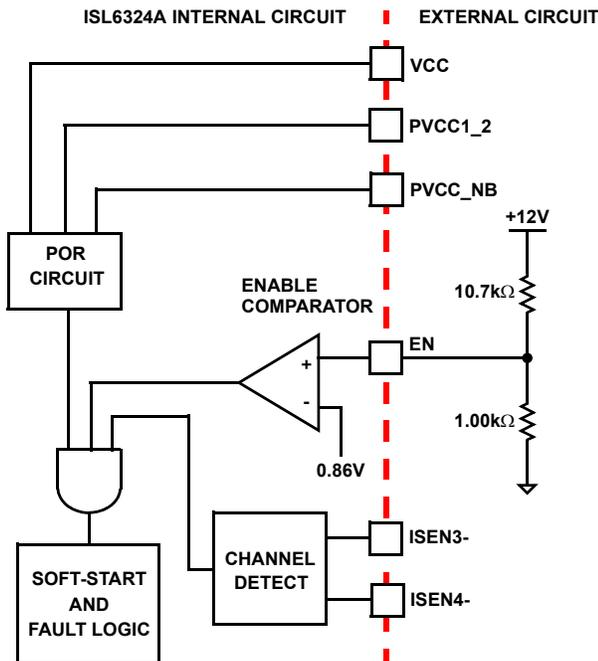
FIGURE 10. POWER SEQUENCING USING THRESHOLD-SENSITIVE ENABLE (EN) FUNCTION
