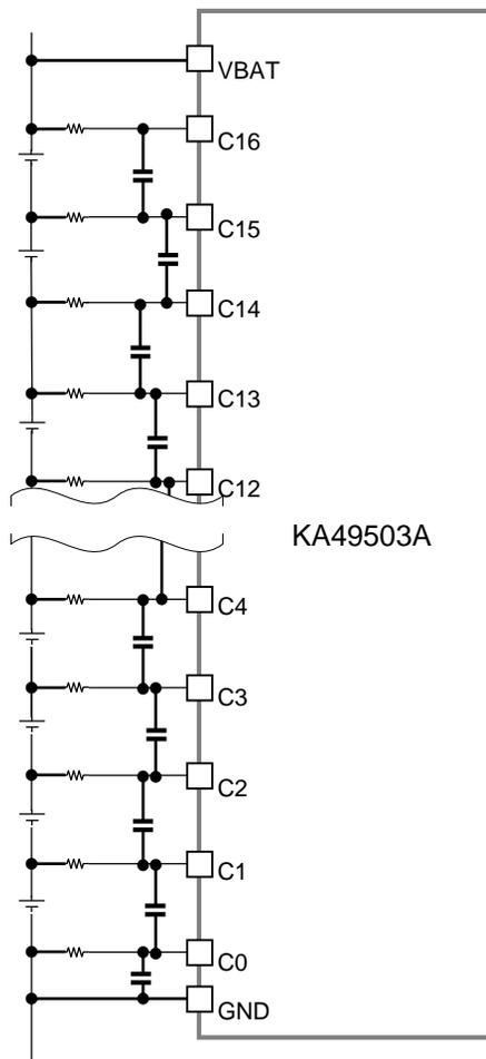
Fig.2.1.1 KA49503A Cell Connection example with 15 cell connected
