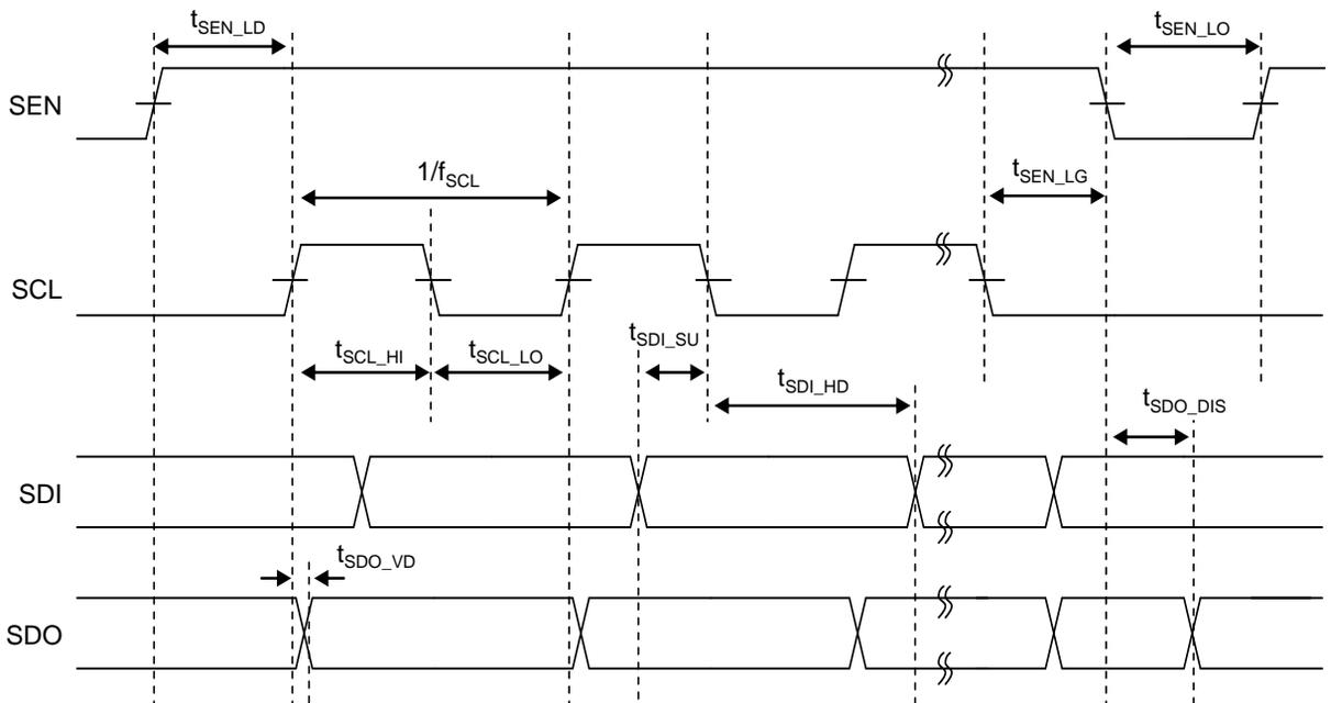
Fig.2.4.1 SPI Timing
