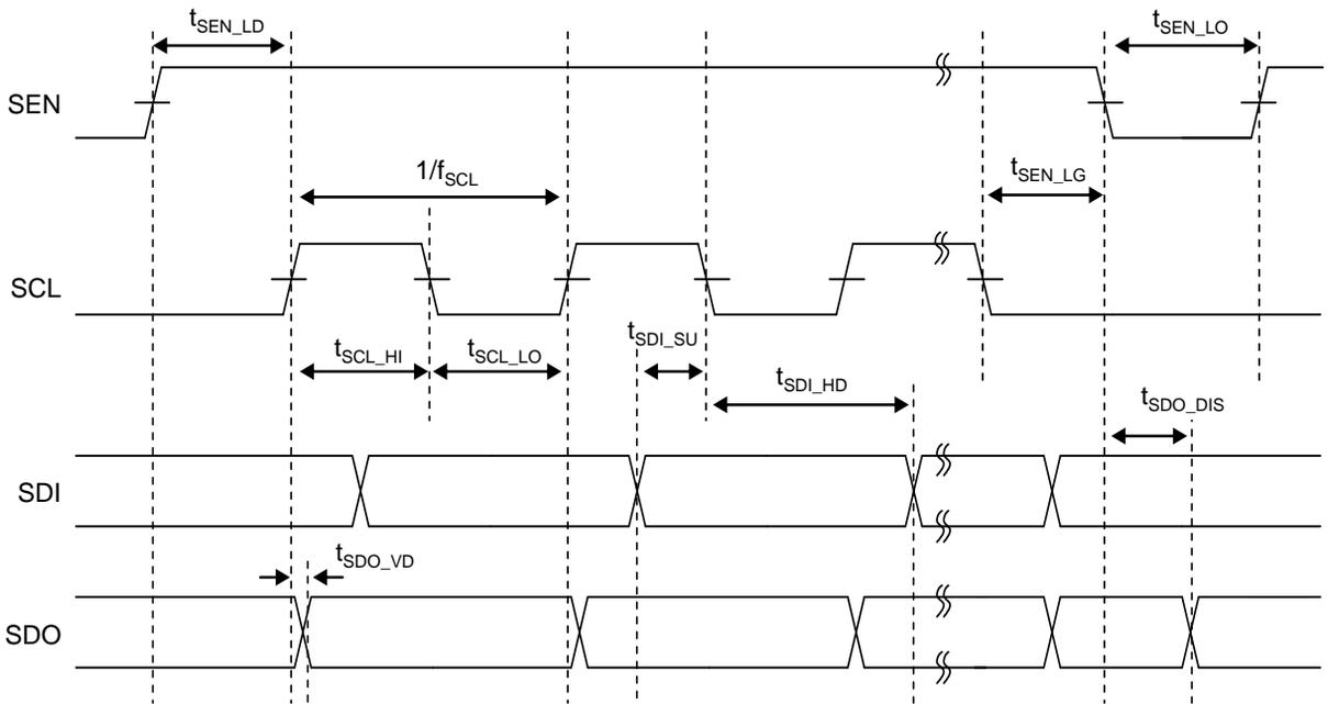
Fig.2.4.1 SPI Timing
