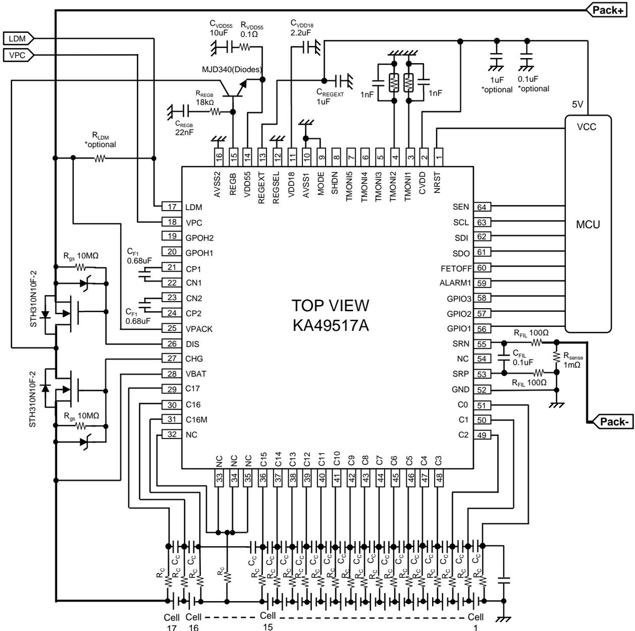
\*1: REGEXT voltage setting can only be set to 5V or 3.3V when using as direct connection with CVDD. There is a requirement for the usage of REGEXT and CVDD total capacitor value. Please refer to page 23 bottom note (\*3) for more detail.
