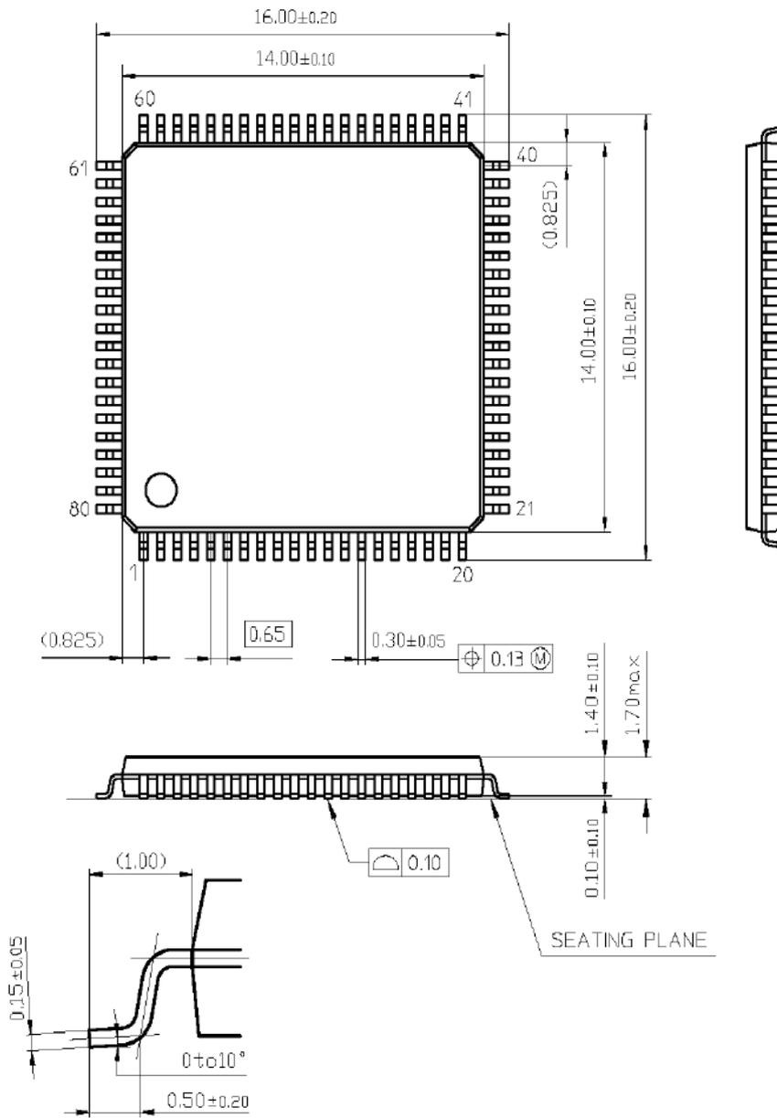
Figure: 6.2 LQFP 80-pin Package Dimension
