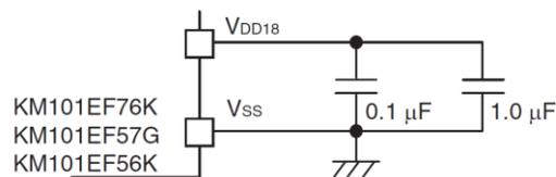
Figure: 5.1 Capacitor Connection between  $V_{DD18}$  and  $V_{SS}$  Pins
