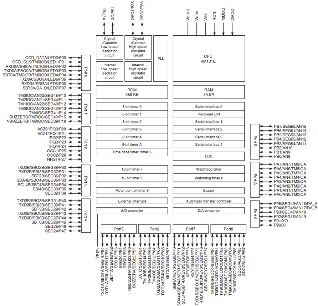
Figure: 4.3 Block Diagram (KM101EF56K)
