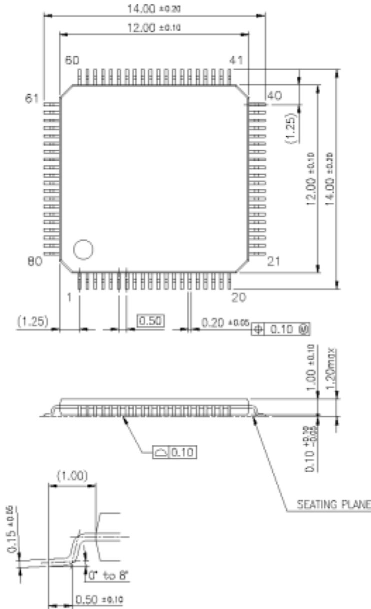
Figure: 6.3 TQFP 80-pin Package Dimension
