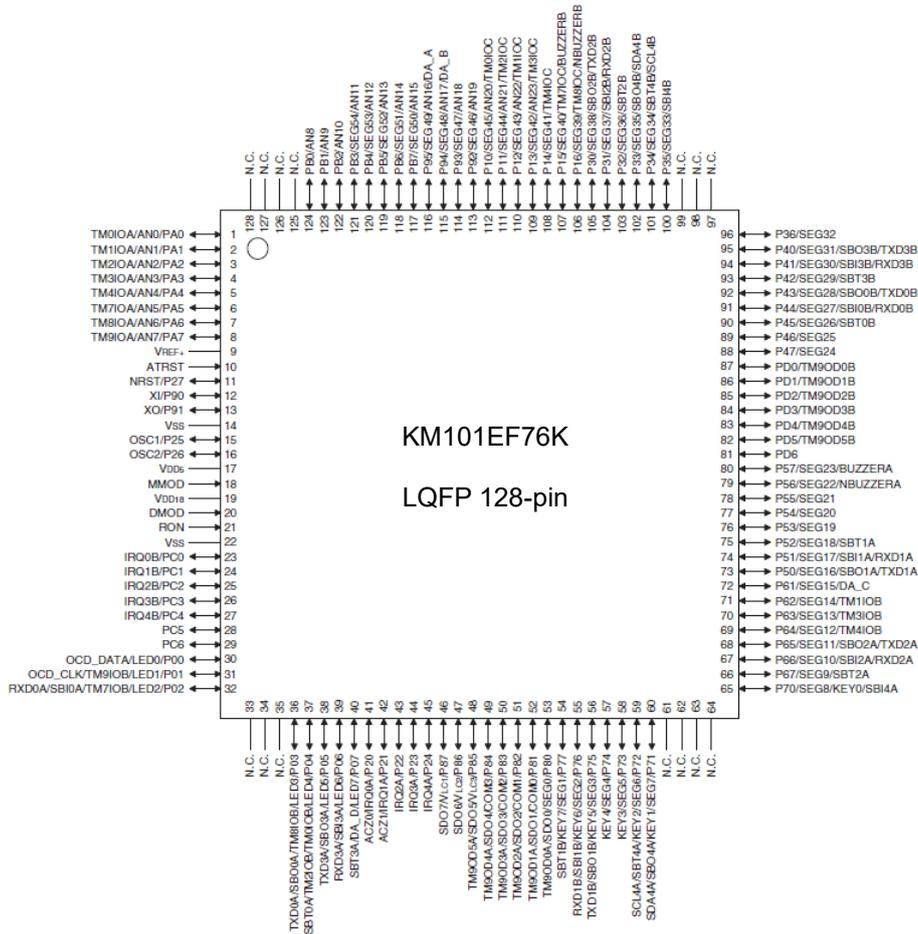
Figure: 3.1 Pin Configuration (KM101EF76K)
