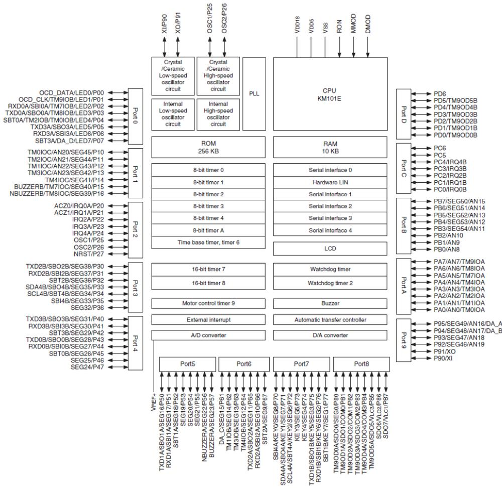
Figure: 4.1 Block Diagram (KM101EF76K)
