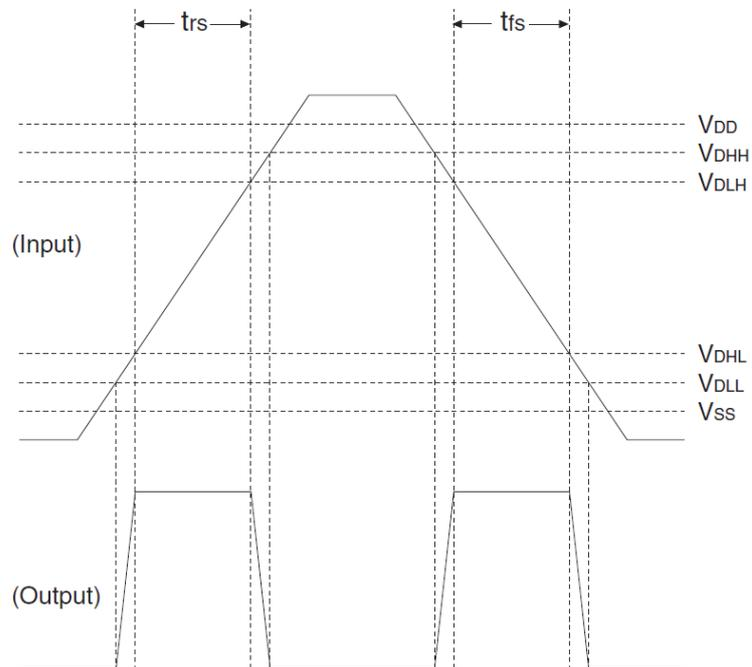
Figure: 5.6 AC zero-volt detection circuit operation
