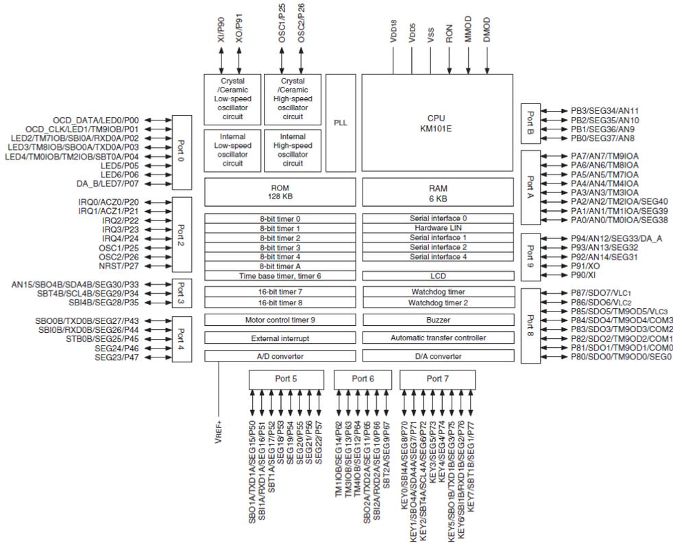
Figure: 4.2 Block Diagram (KM101EF57G)
