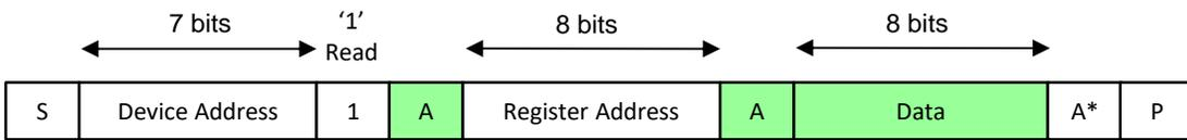
Figure 5. I<sup>2</sup>C Read – Slave Transmitter Mode
