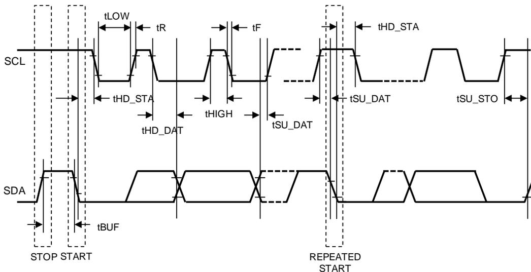
**Figure 2. I<sup>2</sup>C Mode Timing Diagram**
