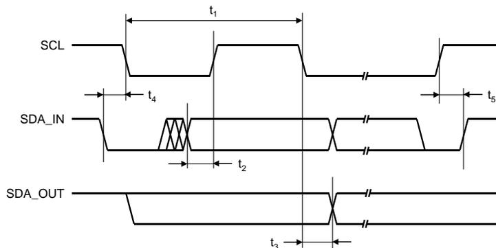
**Figure 1. I<sup>2</sup>C Compatible Interface Timing**
