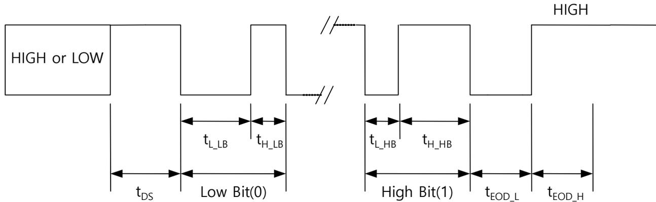
**Figure 5. ExpressWire Interface – Bit Coding Time**
