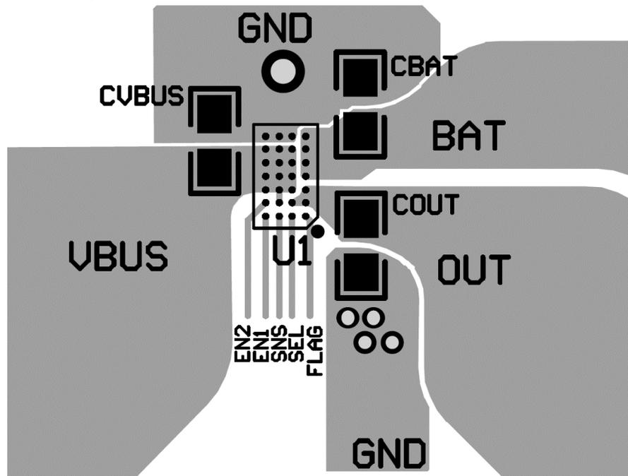
Figure 1. Recommended PCB Layout
