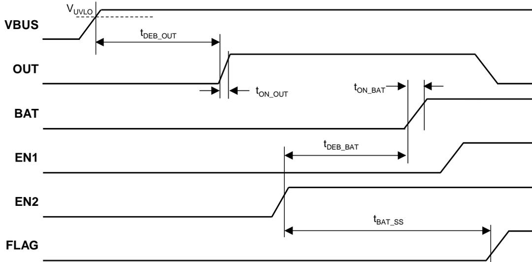
**Figure 5. ON to OFF Timing Normal Operation**
