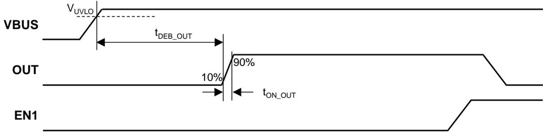
**Figure 1. VBUS to OUT Timing Power Up/Down and Normal Operation**
