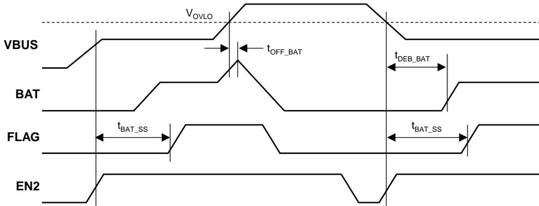
**Figure 4. VBUS to BAT Timing OVLO Operation (EN2 = HIGH)**
