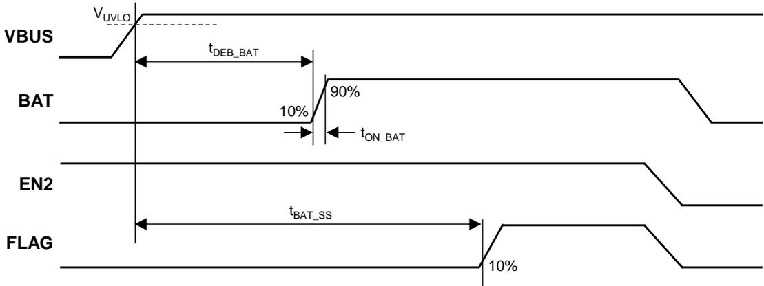
**Figure 3. VBUS to BAT Timing Power Up/Down and Normal Operation**
