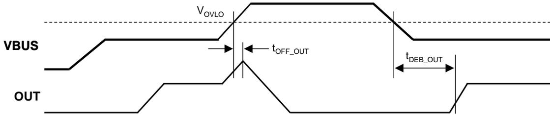
**Figure 2. VBUS to OUT Timing OVLO Operation (EN1 = LOW)**
