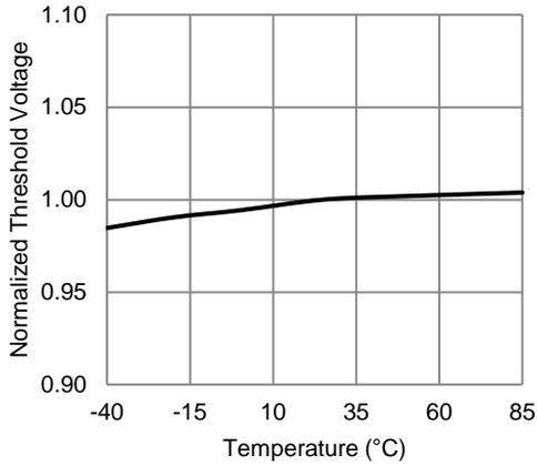
**Normalized VBAT OVLO Threshold vs Temperature**
