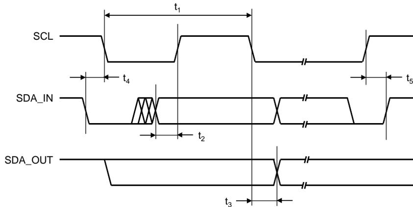
**Figure 2. I<sup>2</sup>C Compatible Interface Timing**
