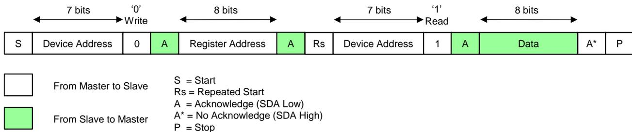
**Figure 5. I<sup>2</sup>C Read Cycle**
