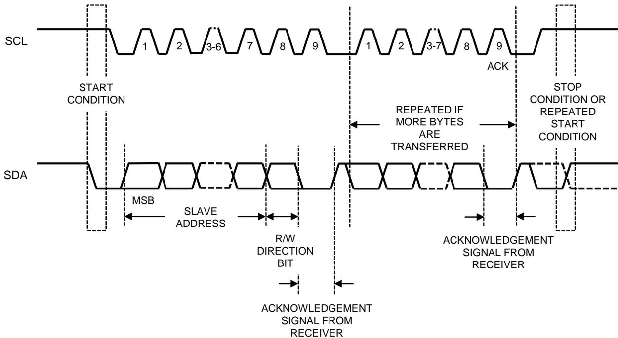
**Figure 3. Data Transfer on I2C Serial Bus**
