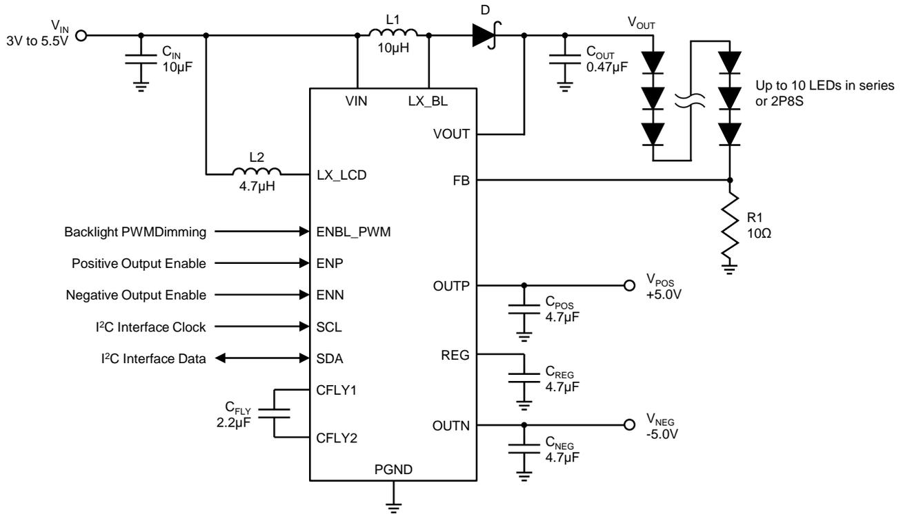
Figure 1. Typical Application Circuit for I<sup>2</sup>C Interface Control
