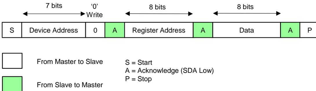
**Figure 4. I<sup>2</sup>C Write Cycle**
