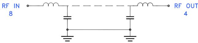
Figure 1. LFCG-360+ Functional Diagram
