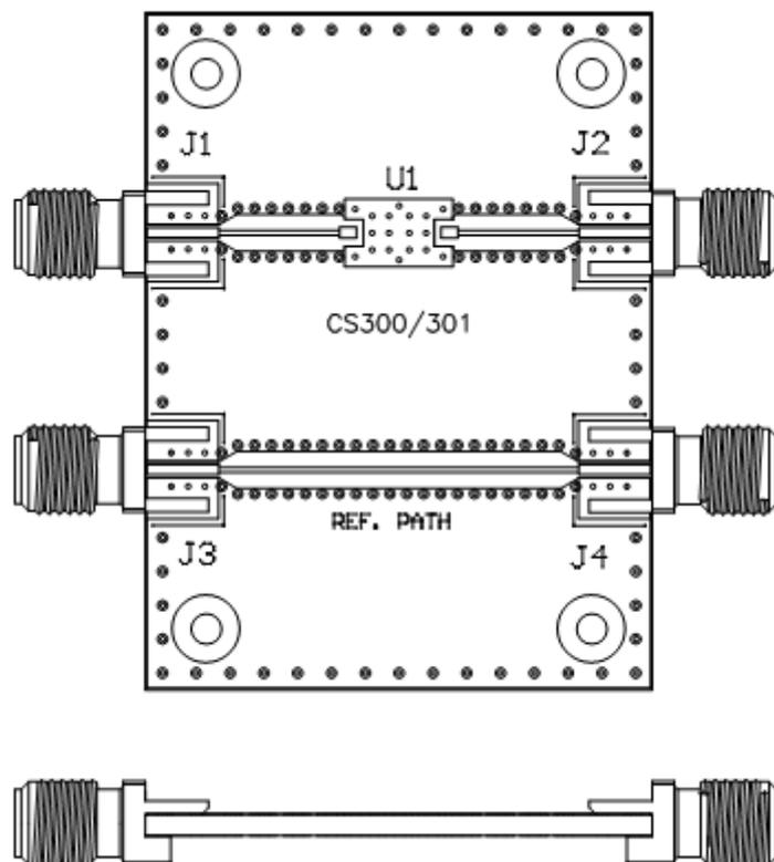
The evaluation board for the LM401102-Q-x-301 is shown above. This evaluation board comprises two sections: the evaluation circuit for the limiter module; and, a reference transmission line.
