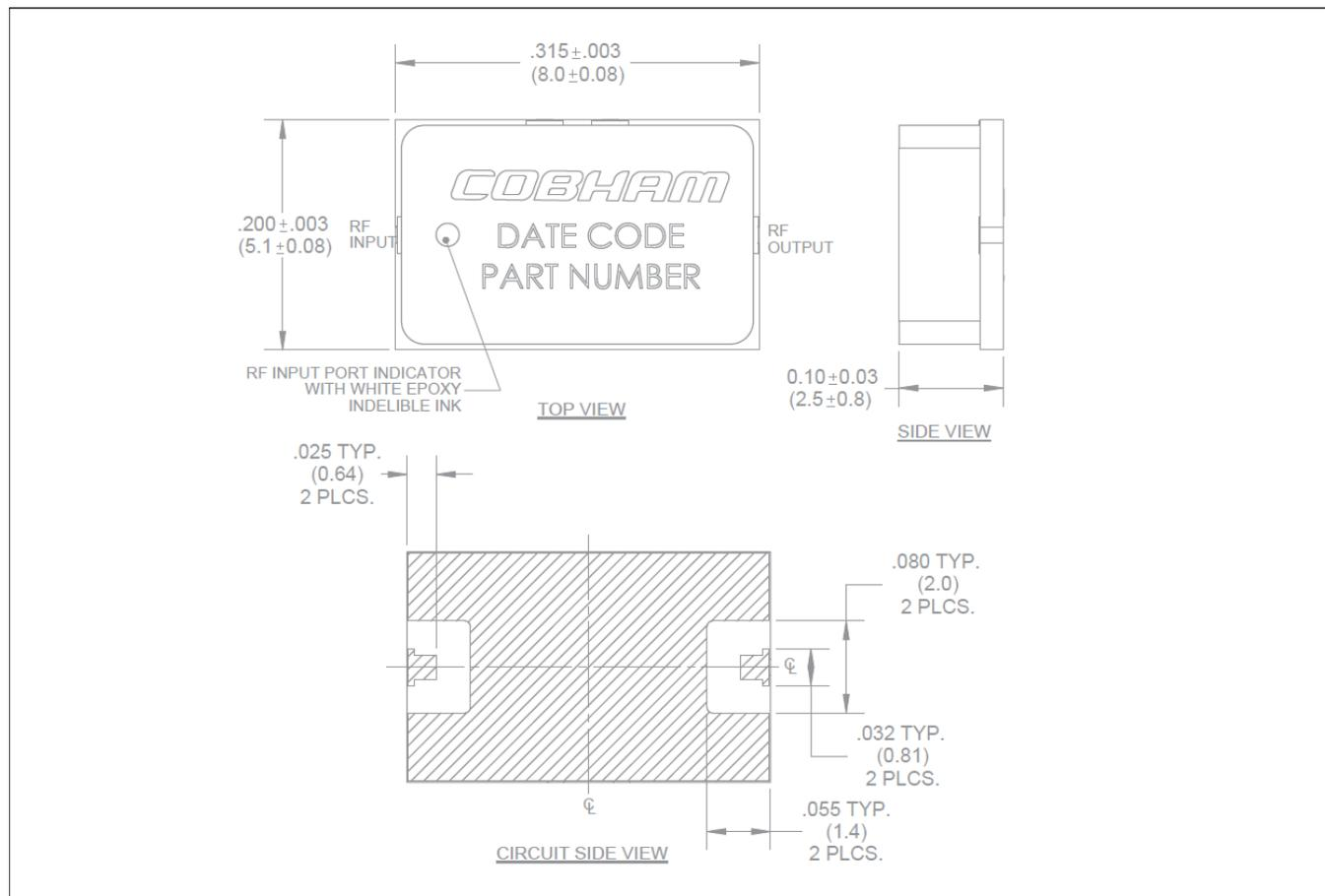
The hatched metal area on circuit side of device is RF and DC grounded.
