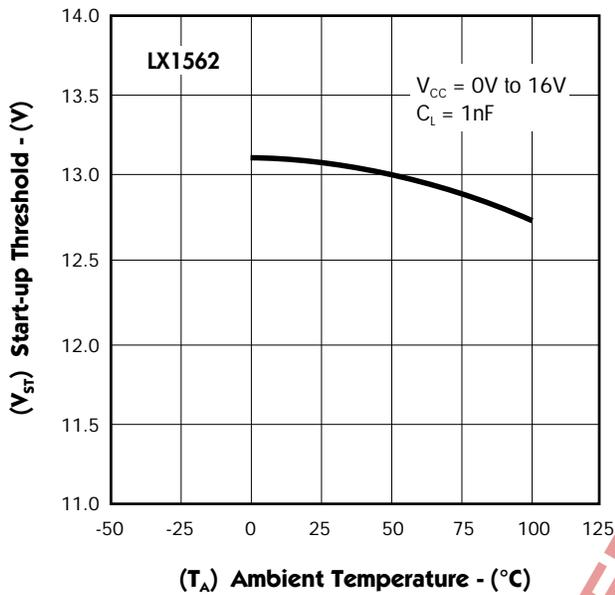
FIGURE 10. — START-UP THRESHOLD vs. TEMPERATURE
