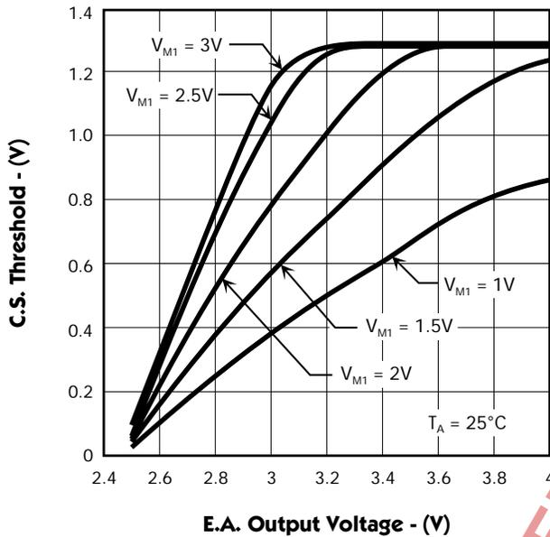
FIGURE 2. — MULTIPLIER INPUT VOLTAGE vs. C.S. THRESHOLD
