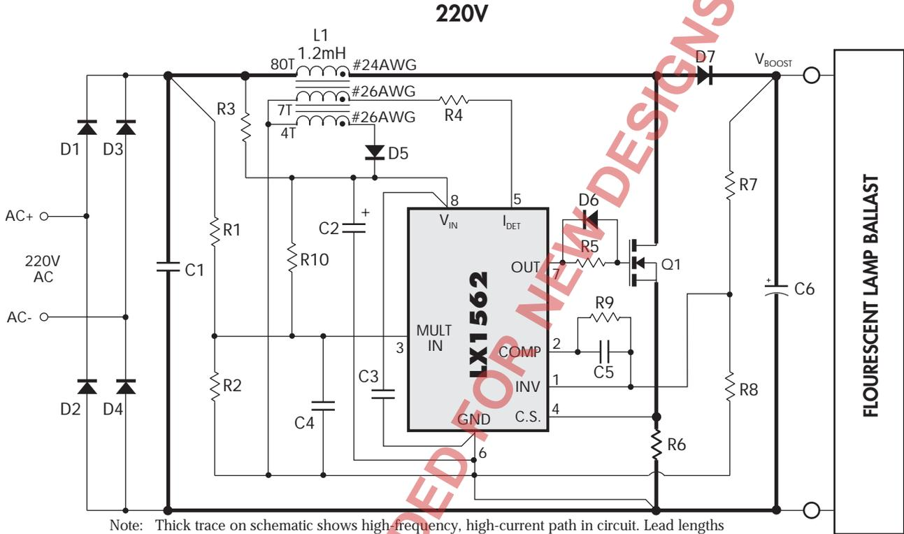
Note: Thick trace on schematic shows high-frequency, high-current path in circuit. Lead lengths must be minimized to avoid high-frequency noise problems.
