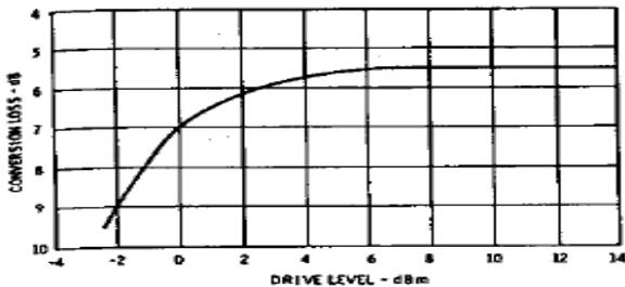
**Conversion Loss vs. Drive Level:** Conversion loss in an SSB system is a function of drive level ( $f_L$  with  $f_L$  and  $f_R$  at approximately 3 GHz and  $f_R$  level at -6 dBm).
