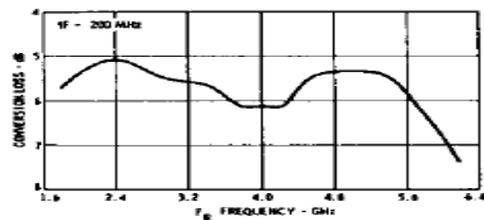
**Conversion Loss vs. Input Frequency:** The frequency ordinate refers to the report ( $f_R$ ) with  $f_L$  at 200 MHz and 1000 MHz, data plotted with  $f_L$  at +7 dBm.
