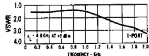
**VSWR vs. Frequency:** VSWR of the L- and R-ports in a 50-ohm system. Some variation in the R-port VSWR will occur as a function of the L-port frequency as shown above. Curves for R-port VSWR are plotted for L-port frequencies of 2 GHz and 4 GHz. A plot of I-port VSWR is also shown with  $f_L$  at 4 GHz.
