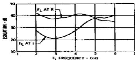
**Isolation vs. Frequency:** Level of the  $f_L$  signal fed through to the R- and I-ports with respect to the level of the  $f_L$  signal at the L-port.
