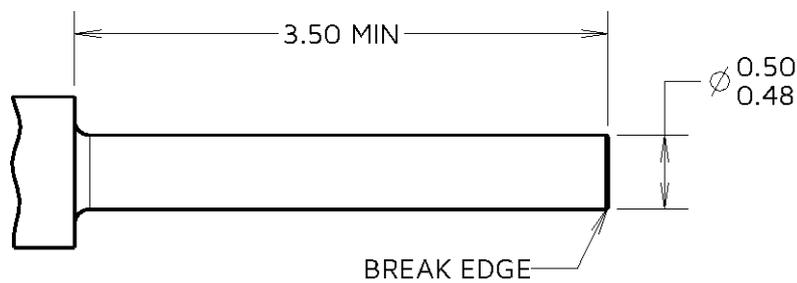
**A3.2. M80 Insertion/Sizing (Pre-Withdrawal) Gauge**
