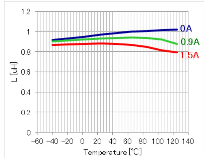
Power Inductors composed of ferrite or metal materials are known to vary their characteristics by temperature and/or DC bias current.
