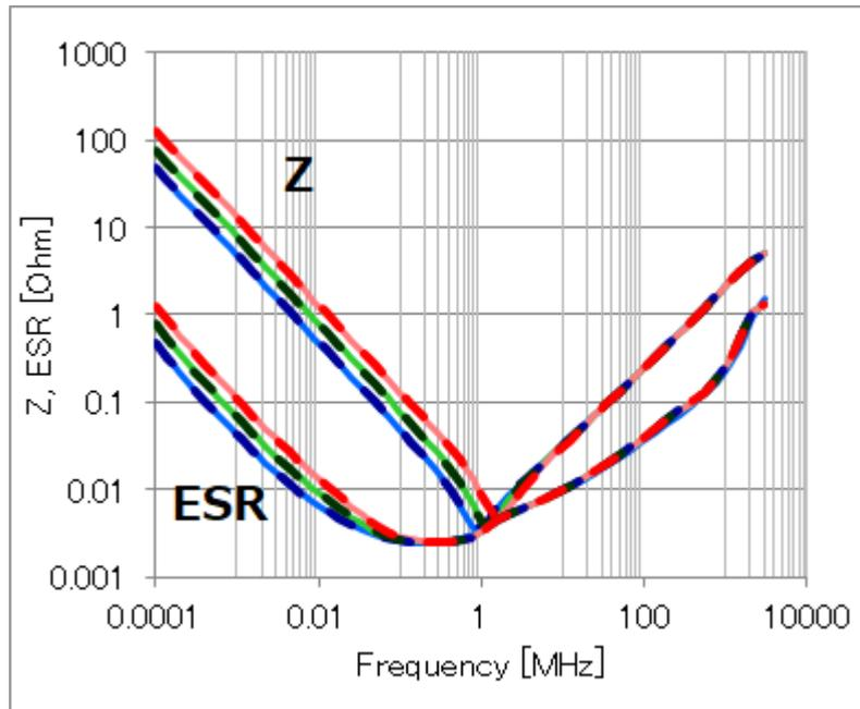
By using Temperature/DC bias model, you can perform simulations well fitting to actual data dependent on the ambient temperature and DC bias current.
