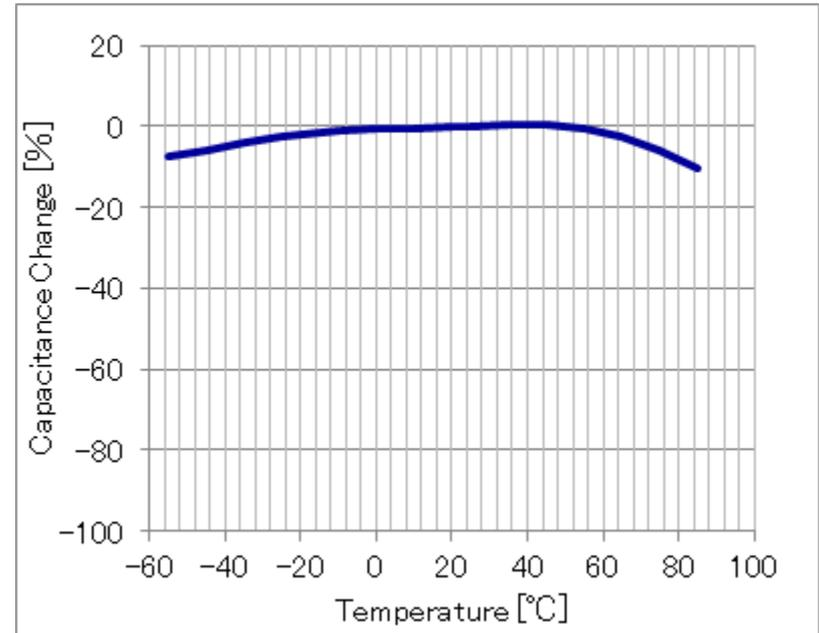
Multilayer ceramic capacitors composed of high dielectric materials are known to vary their characteristics by temperature and/or DC bias voltage.
