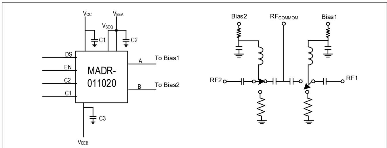
7.  $V_{CC} = +5\text{ V}$  and  $V_{EEB} = -24\text{ V}$ .
