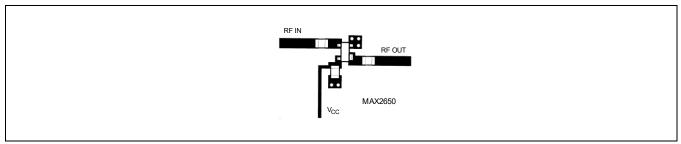
Figure 1. Example PC Board Layout
