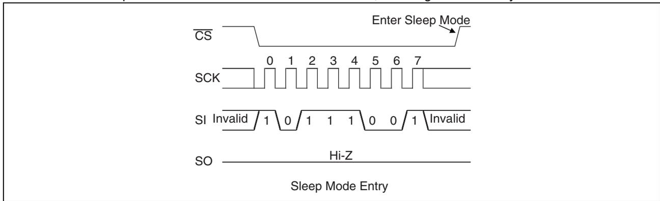
Returning to an normal operation from the SLEEP mode is carried out after  $t_{REC}$  (Max 400  $\mu$ s) time from the falling edge of  $\overline{CS}$  (see the figure below). It is possible to return  $\overline{CS}$  to H level before  $t_{REC}$  time. However, it is prohibited to bring down  $\overline{CS}$  to L level again during  $t_{REC}$  period.
