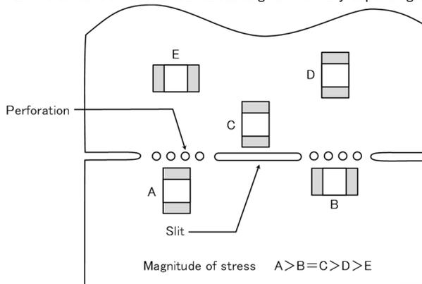
1-3. When PCB is split, the amount of mechanical stress on the capacitors can vary according to the method used. The following methods are listed in order from least stressful to most stressful: push-back, slit, V-grooving, and perforation. Thus, please consider the PCB, split methods as well as chip location.
