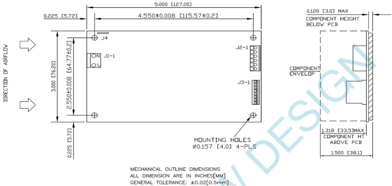
Figure 2. Mechanical Drawing
